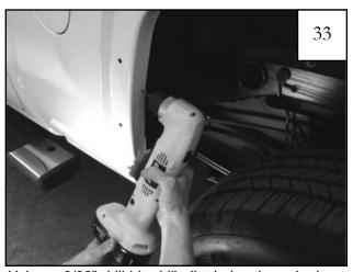
Using a 3/32" drill bit, drill pilot holes through sheet metal at the marks made in Step 30.
