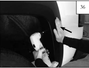
Install self-tapping screws (SW1-0066) into pilot holes drilled in step 31 (3 places). Press flare firmly towards the vehicle while fully tightening.
