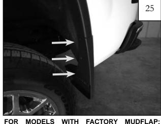
FOR MODELS WITH FACTORY MUDFLAP: Use a Phillips Head Screwdriver to remove 3 factory mud flap fasteners.
