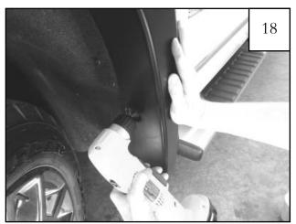
Install self-tapping screw (SW1-0066) into pilot hole drilled in step 15. Press flare towards vehicle while fully tightening. *Note: This step not needed for models with factory installed mudflaps.*
