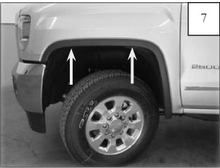
Remove two fasterners along top of factory wheel arch molding using a T-15 Torx bit.
