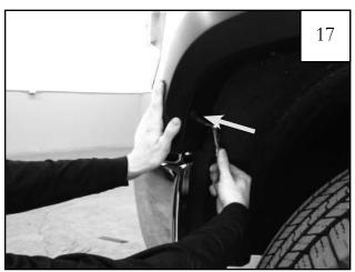
While holding Flare on vehicle, install factory screw removed in Step 6 through flare and into factory hole. Do not fully tighten at this time.
