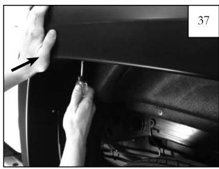
Press flare towards vehicle and fully tighten all remaining fasteners.
