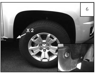
Using a T-15 torx bit, remove two factory fasteners from mud guard. Discard factory fasteners only..
