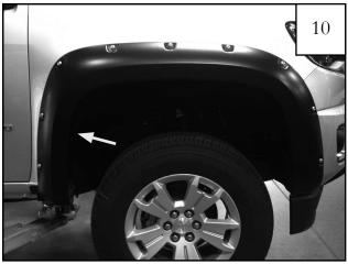
Holding the flare into position on vehicle, use a grease pencil or sharple to mark sheet metal using the upper rear hole location as a guide.
