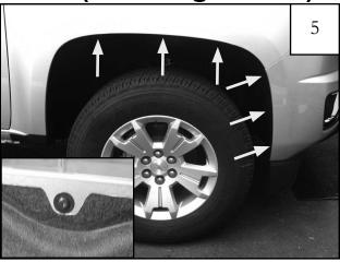
Using a T-15 torx bit, remove six factory fasteners from wheel well. Retain for bracket installation.
