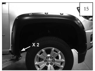
Start two supplied screws (SW1-0056) into the two botton rear mounting locations. Fully tighten all screws.
