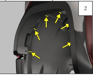
While holding the front flare in place, mark the flare's (6) hole locations using a grease pencil. (Wheel only removed for visual clarity.)
