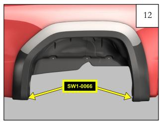
Using an electric drill/driver, install rear flare using (2) SW1-0066 drill screws through the sheet metal flanges at the bottom of the fender.
