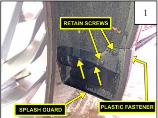
Remove the front splash guard using a T-15 Torx driver and retain (2) screws for later use.
