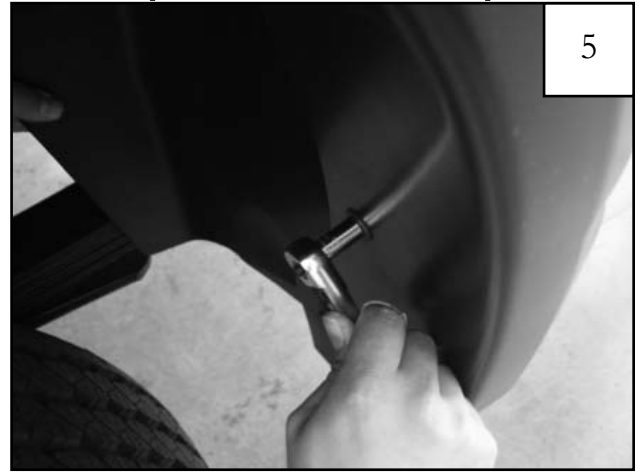
Holding flare in position on fender, reinstall screws removed in Step 4. Do not tighten. (An awl may be used to align the threaded clip with holes in flare and fender lip) Note: Make sure screws engage in splash shield.
