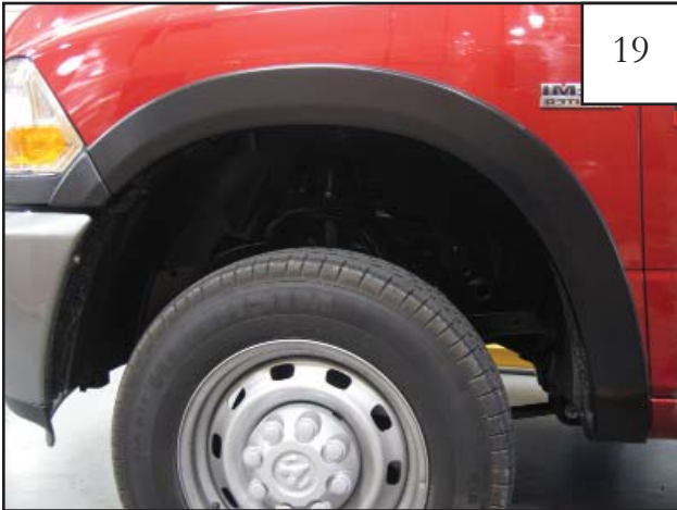
Completed front flare installation.
