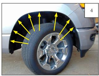
Remove and keep (8) factory installed screws. The remaing screws will be re-used to install the front flare.
