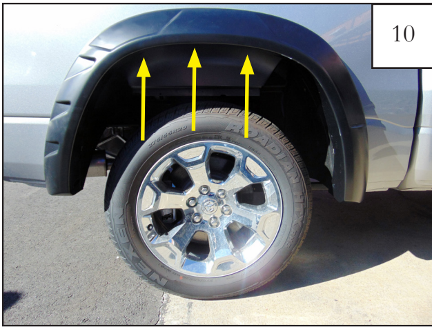
Hold flare in place and reinstall (3) factory screws removed in Step 9. Do not tighten.
