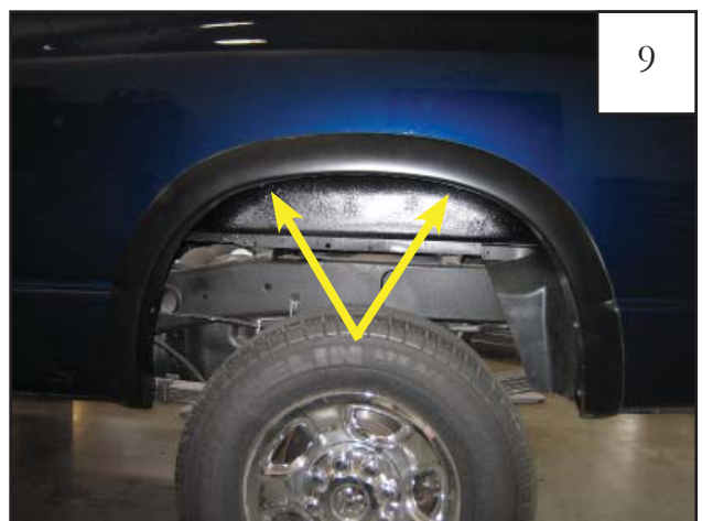
Long Clip locations. Note: Clips will be offset of fender to allow for screw to tighten.
