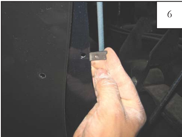
Slide a supplied Small Clip over fender lip at front of wheel well, aligning with existing holes in fender (2 places).
