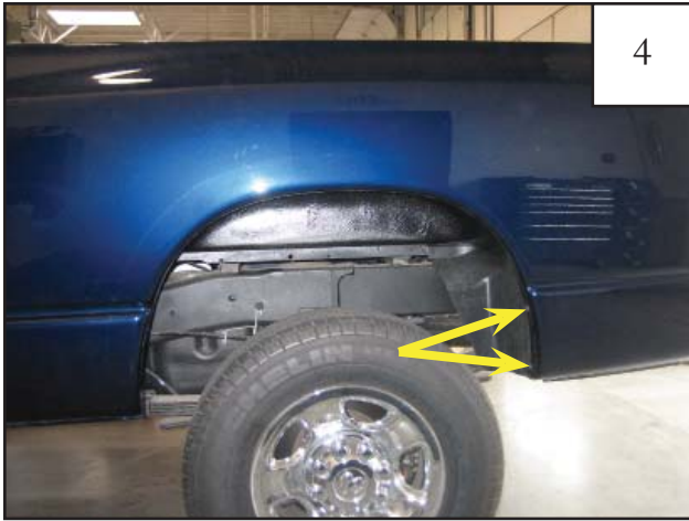
Using an 8mm socket, remove two factory screws from rear of wheel well. Retain for future use.
