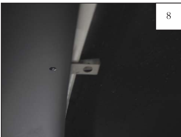
Slide a supplied Long Clip onto top of fender well, aligning with holes in the flare (2 places). (There are no factory holes at these locations.)
