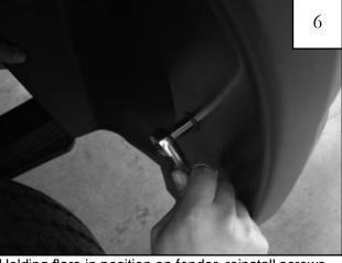
Holding flare in position on fender, reinstall screws removed in Step 5. Do not tighten. (An awl may be used to align the threaded clip with holes in flare and fender lip) *Note: Make sure screws engage in splash shield.*
