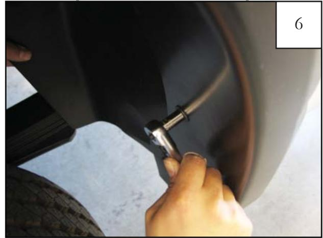
Holding flare in position on fender, reinstall screws removed in Step 5. Do not tighten at this time. *Note: An Awl may be used to align the threaded clip with holes in flare and fender lip. Make sure screws engage in splash shield.*
