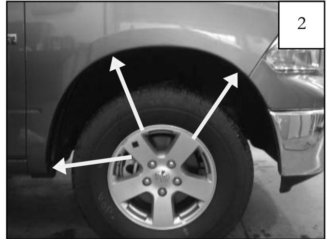
Remove three factory installed screws with 8mm socket wrench.
