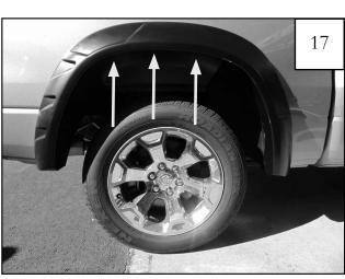
Hold flare in place and reinstall (3) factory screws removed in Step 16. *Do not tighten*.
