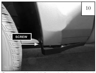
Remove and keep (1) factory installed screw, and remove mud flap from vehicle. This factory screw will be used to install the rear fender flare.
