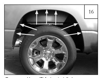
Remove and keep (7) factory installed screws.
