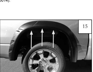
Hold flare in place and start Screw (SW1-0056) using a Phillips screwdriver in (3) locations as shown. *Do not tighten.* **Continue to Step 18.**
