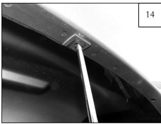
Using an awl or similar pointed tool, poke a hole through Tab (MT1-0014) using the Clip (CL1-0022) hole as a guide. Repeat Steps 12-14 for remaining (2) empty hole locations.
