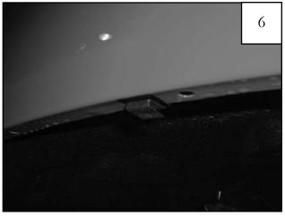
Slide the supplied "S" Clips over the Plastic Tabs on the fender lip (3 places).
