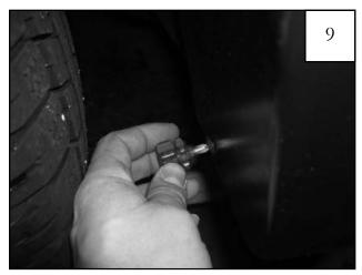
Hold the flare on the fender. Start a supplied #8 Truss-Head Screw through the lower rear hole in the flare and into the "U" Clip installed in Step 8.
