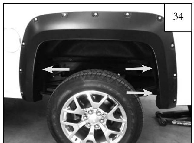
Hole locations to be marked for drilling.
