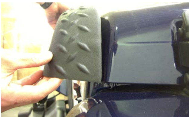
Photo #5 – Hood Protector placement
