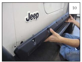
Gently position part on vehicle, centering between fender flares (about 1/4" to 3/8" space on each side). Take care not to press the part onto vehicle until properly positioned.
