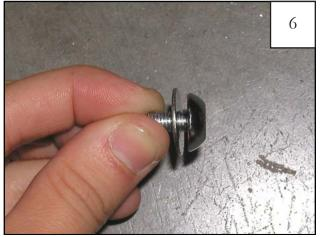
Slide a supplied washer (WA1-0007) onto a supplied screw (SW1-0032).
