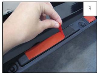
Remove red vinyl backing from tape pads. NOTE: Check part for engraved "14008R" or "14008L" prior to proceeding to the next step. The left part will go on the driver's side.
