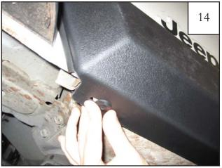
Attach underside edge of the Rocker Panel to the vehicle using supplied Tuflocs fasteners (RV1-P001), pressing Tuflocs through slots and into factory holes.
