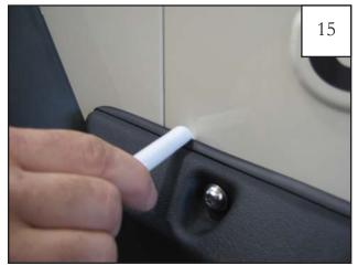
Using supplied Edge Trim Tool, seat top edge of edge trim first by hooking curved end under top edge at one open end and slide over entire top edge to the other end.
