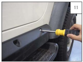
Once part is positioned, press firmly on screw heads to adhere inner pieces to vehicle. Remove screws and remove outer part from vehicle, leaving the inner pieces on the body.
