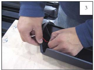
Applying the adhesive side of the edge trim (GP1-0005) to the inner side of part, affix edge trim to the top edge of the part (the portion that comes in contact with vehicle).
