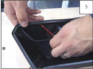
Press edge trim (GP1-0005) into place along the top edge of the flare in one foot increments, pulling red vinyl backing free as you go.
