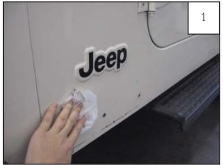
Wipe side of vehicle with alcohol wipe to remove grease and dirt.
