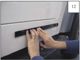
Apply 30 pounds of pressure per square inch to the inner pieces to ensure proper tape adhesion.
