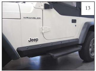
Reinstall part as shown in Step 8, taking care that screws are snug. Do NOT overtighten, as the screws may strip out.
