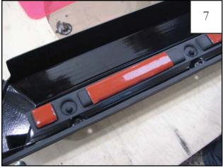
Align three indents in each taped inner piece with three holes in parts. Tape attached to inner pieces should be facing away from the inside of the part.
