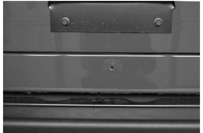
Figure #4 – Remove Tire Stop
