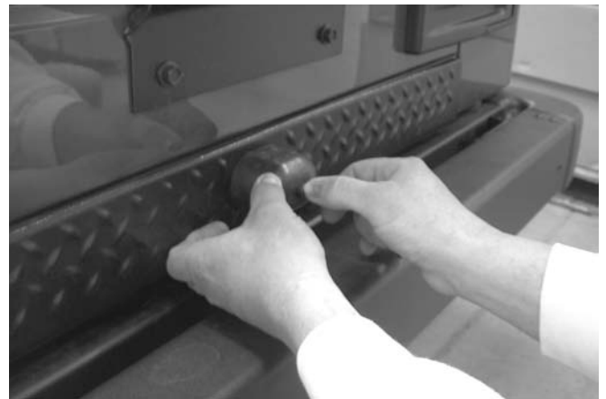
Figure #5 – Reinstall Tire Stop & Tire
