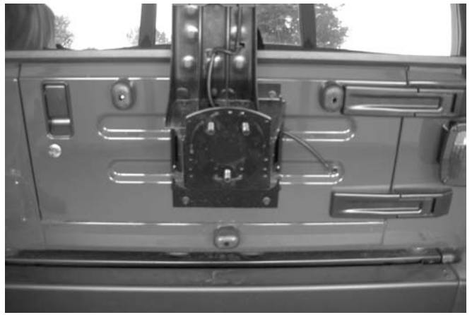
Figure #3 – Remove Spare Tire
