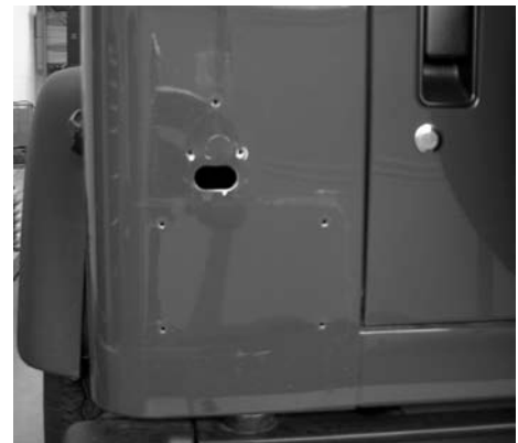
Figure #2 – Remove Tail Light & License Plate
