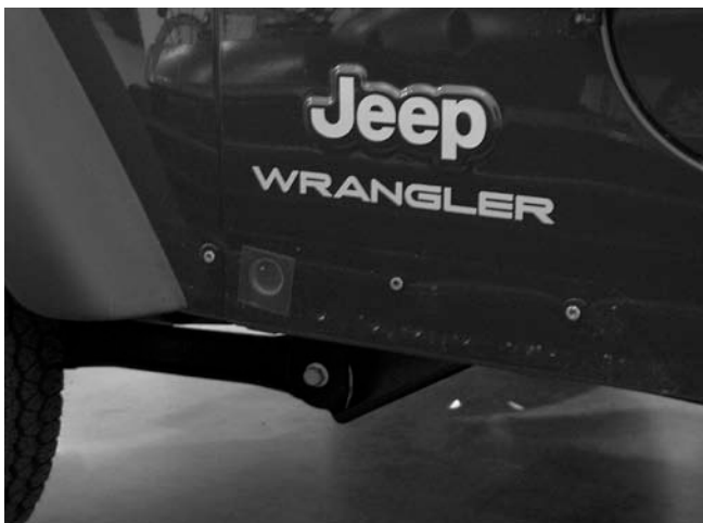
Figure #6 – Remove Stone Guard
