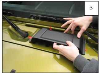
Hold the part at an angle to prevent tape from prematurely sticking, and align the part on the hood using marks made in Step 3 as a guide. NOTE: *If necessary, lift windshield wiper out of the way.*
