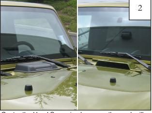
Center the Hood Scoop in place over the cowl grille in desired orientation.
