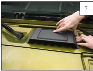
Press part into place. Apply 30 PSI to the taped areas for proper bond. The tape reaches maximum adhesive bond after 24 hours of contact. Do not wash vehicle for 24 hours.
