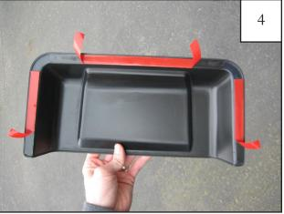
Remove part and peel red liner partially from tape pads as shown. NOTE: *Make sure tabs are folded toward the outside of the part and are accessible to pull once part is repositioned.*
