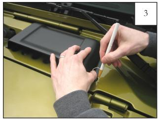
Once positioned, use a grease pencil to lightly trace around edges of part.
