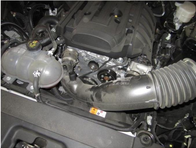
9. Remove the factory intake ducting from the engine compartment.
