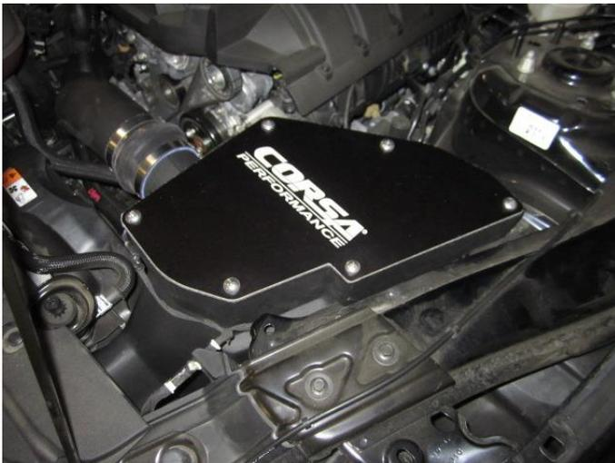
23. Attach the CORSA air box lid using the provided truss head screws and rubber washers. Check all connections and clamps before starting the vehicle. Reattach the negative battery cable and retighten all connections after 100, 500 and 1000 miles. **Reconnect the battery cable**
