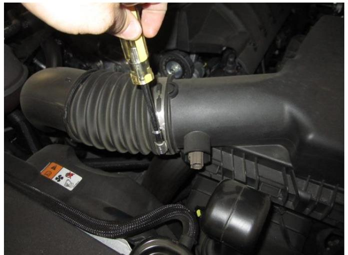
4. Loosen the clamp holding the duct to the air box.
