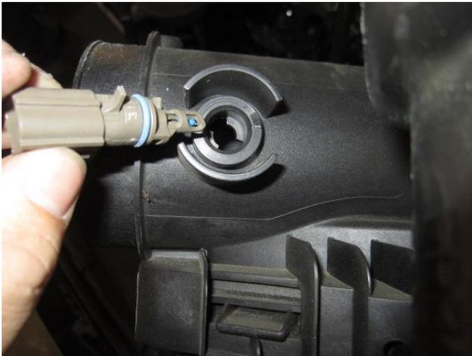
11. Remove the ATS sensor from the air duct.
