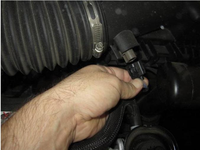
1. Disconnect the ATS sensor harness from the ATS sensor.
