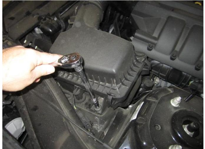
2. Remove the 10mm bolt holding the factory air box in place.
