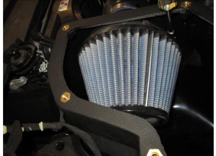
22. Attach the 5120 Ram filter onto the filter adapter using a 5/16 socket or nut driver only.
