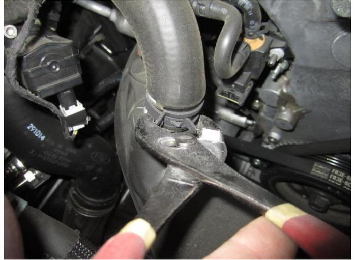
6. Using a pair of pliers remove the blow off valve hose from the factory intake duct.
