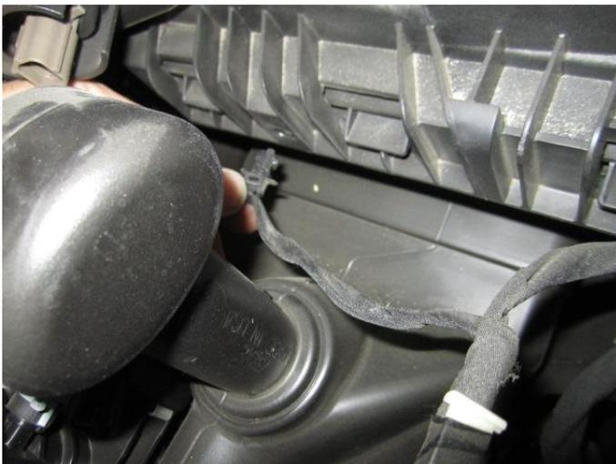
3. Remove the ATS sensor harness from the factory air box.
