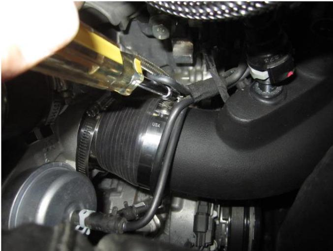
19. Tighten the reducer to the CORSA duct with the #48 clamp using a 5/16 socket or nut driver only.
