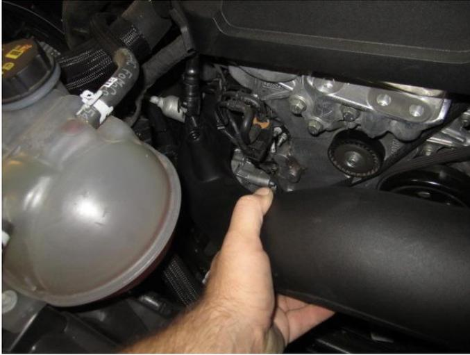
17. Slide the CORSA duct into the reducer but do not tighten the clamp at this time.
