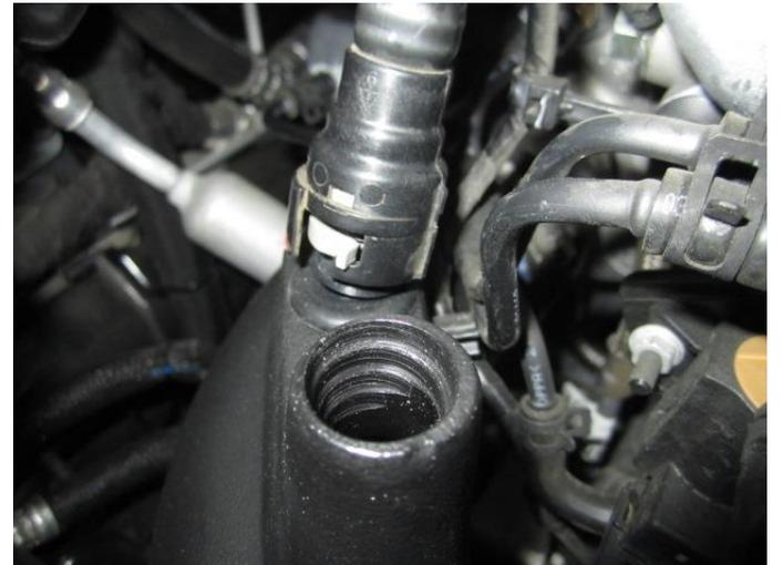
20. Attach the crankcase vent hose onto the supplied 5/8 snap fitting.
