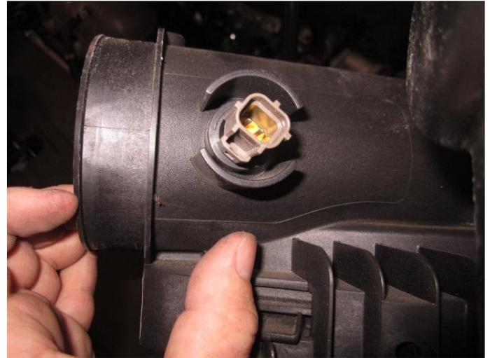
10. Lift the tab on the ATS sensor and rotate counter clockwise.
