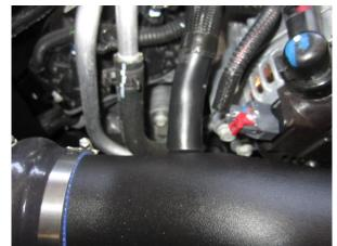
**10.** Install factory breather hose onto air duct.
