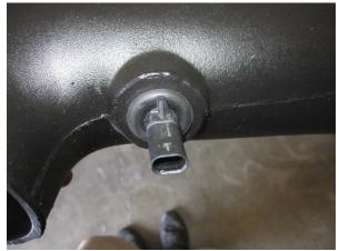
Locate the CORSA air duct. Push the air temperature sensor into the CORSA air duct.
