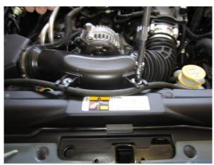
**3.** Remove the two bolts securing the factory air duct to the core support using a ratchet and 10mm socket.
