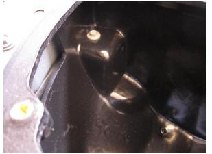
2. Locate bolt removed in removal step 10 and use it to secure air box into place. Tighten bolt using a ratchet and 10mm socket.
