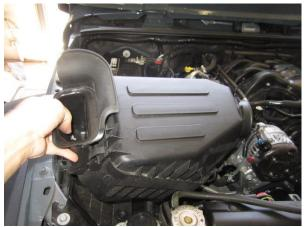
**9.** Remove the factory air box by pulling up.
