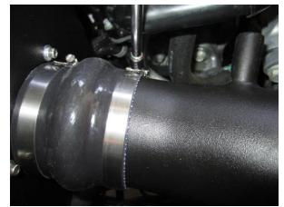
**9.** Tighten clamp on hump hose using a flathead screwdriver or ratchet and 10mm socket.
