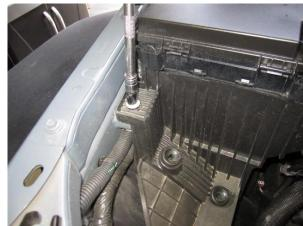
Remove the bolt in front of the fuse box using a ratchet and 10mm socket.
