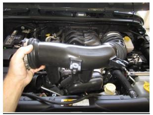
**1.** Remove the factory air duct from vehicle.
