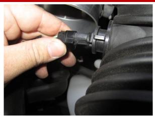
**6.** Disconnect the wiring harness from the ATS sensor on factory air duct.
