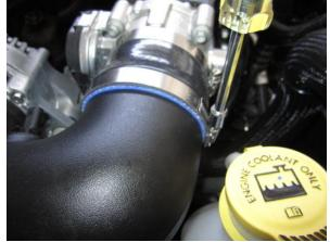
8. Install air duct into hump hose and straight sleeve. Adjust duct as necessary and tighten clamp on straight sleeve using a flathead screwdriver or ratchet and 10mm socket.
