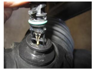
Locate the factory air duct and remove the air temperature sensor by gently lifting tab and twisting counterclockwise then pulling straight out.
