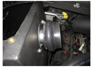
**8.** Locate the Ø4.0" Hump Hose and one #64 clamp. Install the hump hose and clamp onto the filter adapter and snug clamp to hold hump hose in place. Do not fully tighten.
