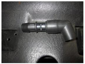
**1.** Locate the supplied 3/4" straight fitting and the factory breather hose elbow from removal step 6 and install the fitting into the factory elbow.
