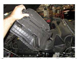
Remove the factory air box by pulling the air box straight up and off of the grommet posts.
