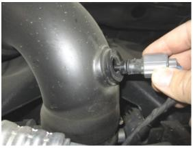
Disconnect the ATS sensor harness from the sensor and remove it by twisting and pulling straight out.
