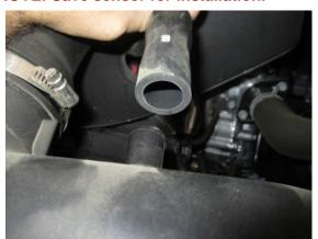
**3.** Disconnect factory breather hose from factory air box by pulling straight out.
