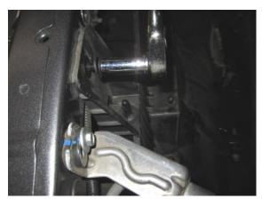
Remove the two 13mm air box mounting tray bolts securing the tray to the inner fender.
