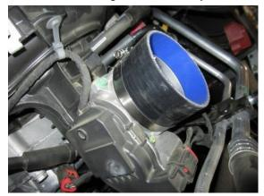
**3.** Locate the Ø3.5"x2.5" straight sleeve and one #56 clamp and install the straight sleeve with clamp onto the throttle body. Snug clamp to hold straight sleeve in place, but do not fully tighten.
