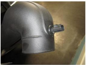
9. Locate the ATS sensor from removal step 1 and the CORSA air duct and install the sensor into the ½" grommet on the air duct paying attention to the direction of the sensor.
