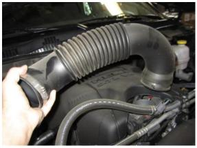
2. Loosen the clamps securing the factory air duct to the throttle body and factory air box using flathead screwdriver or ratchet with 8mm socket. Remove factory air duct from vehicle.
