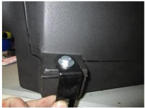
**5.** Locate the longer L-bracket, one 6mmx25mm bolt, flat washer, lock washer, and 6mm nut and install bracket to front side of box closest to headlight.
