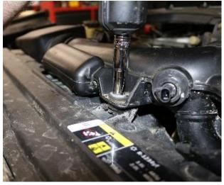
Remove the two bolts securing the factory air duct to the core support with a ratchet and 10mm socket.
