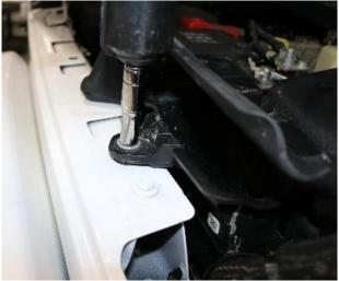
Remove the bolt securing the factory air box to the inner fender with a ratchet and 10mm socket.NOTE: Save bolt for installation.
