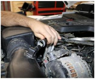
6. Disconnect the breather hose from the factory air duct by squeezing gray tab and pulling straight off.
