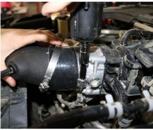
10. Adjust air duct as necessary and tighten all four clamps using a flathead screwdriver or ratchet and 8mm socket.
