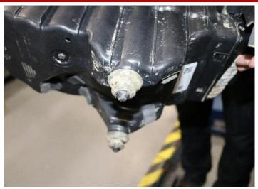
Remove the two mounting grommets from the bottom of the factory air box.
