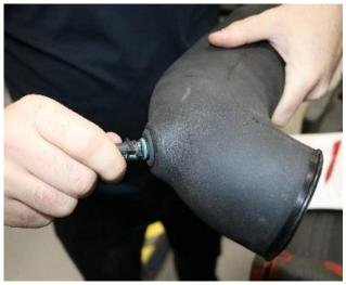
Locate the air temperature sensor from removal step 10 and CORSA air duct and install the sensor into the air duct
