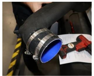
**1.** Locate the CORSA air duct, Ø3.25" straight sleeve, and two remaining #56 clamps. Install straight sleeve and one #56 clamp onto air duct and snug clamp to hold straight sleeve in place. Place the other clamp onto straight sleeve.
