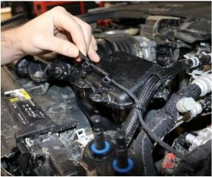
Using a trim removal tool, remove the two clips securing the ATS wiring harness to the factory air duct.
