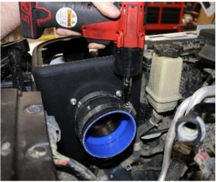
**6.** Locate the Ø3.5" Hump Hose and two of the #56 clamps. Install the hump hose and one #56 clamp onto to filter adapter. Snug the clamp to hold the hump hose in place, but do not fully tighten. Place the other clamp onto hump hose.
