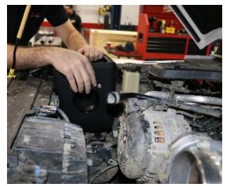
4. Locate the CORSA air box and install into vehicle by fitting the posts on the bottom of air box into the factory grommets installed in step 1.
