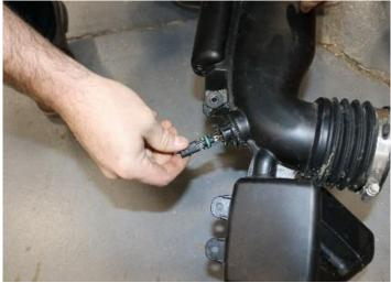
10. Remove the air temperature sensor from the factory air duct. Pay attention to the orientation of the sensor prior to removal to aid in installation. NOTE: Gently lift tab to clear locking feature and rotate sensor approximately one quarter turn counterclockwise until it stops. Pull sensor straight out.
