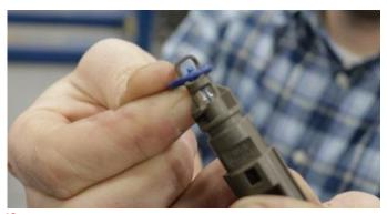
**10.** Remove O-ring from the temp sensor.
