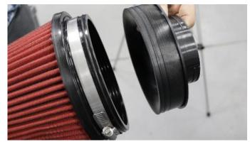
**10.** Locate filter and filter adapter and insert the filter adapter into filter. Tighten clamp enough that it won't fall off filter but leave loose enough to rotate.
