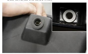
**5.** Locate the CORSA air box, and the factory grommet and metal bushing from Removal Step 7 and install grommet in air box then the metal bushing into grommet from inside box.
