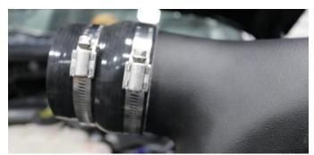
**16.** Locate reducer, #56 clamp and #48 clamp. Install large end of reducer and # 56 clamp onto upper outlet of air duct. Tighten clamp using a flathead screwdriver or ratchet and 8mm socket. Loosely place #48 clamp onto reducer.
