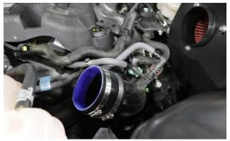
15. Locate straight sleeve and remaining two #64 clamps. Install straight sleeve and one #64 clamp onto driver side turbo inlet tube and tighten clamp using a flathead screwdriver or ratchet and 8mm socket. Loosely place other #64 clamp onto straight sleeve.
