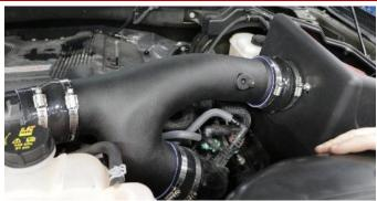
**18.** Adjust air duct as necessary and tighten all clamps using a ratchet and 8mm socket or flat head screwdriver.
