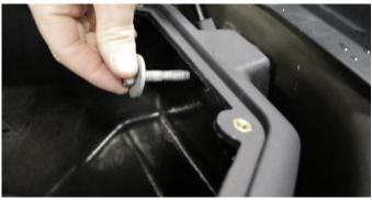
8. Locate the bolt from removal step 4 and attach the CORSA air box to the inner fender using a ratchet and 13mm socket.
