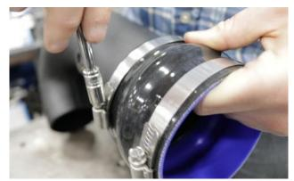
14. Locate the hump hose and two # 64 clamps. Install the hump hose and one clamp onto the air duct inlet end and tighten clamp using a flathead screwdriver or ratchet and 8mm socket. Loosely place other clamp on hump hose.
