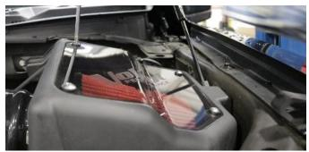
Locate CORSA lid assembly and four lid screws with rubber washers. Install lid using Philips head screwdriver.
