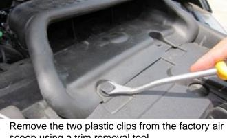
scoop using a trim removal tool. **NOTE: Save clips for installation.**
