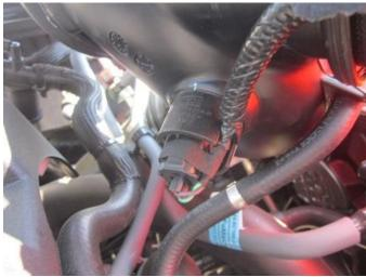
Disconnect the wiring harness from the air temperature sensor on back side of factory air duct.
