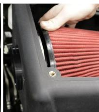
11. Insert the filter into the air box with the adapter side down. Rotate the top of the filter down into the air box and rotate the filter around and push the adapter through air box.
