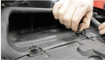
Locate the air scoop retaining clips from removal step 6 and attach factory scoop.
