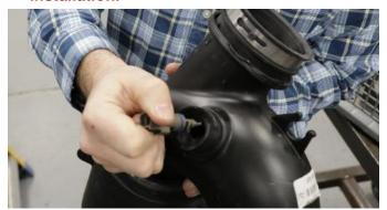
Remove the air temp sensor from factory duct by gently lifting tab and rotating counterclockwise until it stops then pulling straight out. NOTE: Save for installation.
