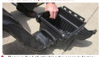
**8.** Remove the bolt attaching the scoop to factory air box using a ratchet and 8mm socket. Remove the factory air scoop from the bottom of the air
