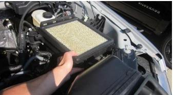
Remove the bottom box assembly by pulling it up and out. Remove the rubber grommet and metal bushing from factory air box to inner fender mounting location.
