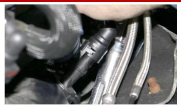
Unclip the quick disconnect vent hose on the driver side turbo inlet tube.
