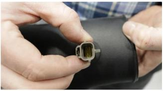
13. Locate air temperature sensor from removal step 9 and CORSA air duct. Install sensor into grommet with tab facing the closest end of air duct.
