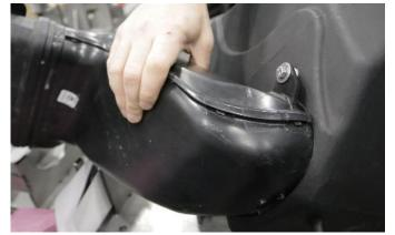
Locate the 6mm x 25mm bolt. .25" x .75" flat washer, one .25" x .63" flat washer, one .25" lock washer, 6mm nut, .25" spacer, and factory air scoop from removal step 8. Attach air scoop to air box placing the spacer between the scoop tab and air box. Tighten hardware with 10mm wrenches.
