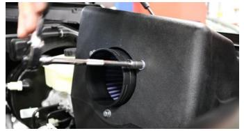
6. Locate three 6mm x 16mm bolts, three remaining .25" x .63" flat washers, and three remaining .25" lock washers. Attach filter adapter to air box and tighten using a ratchet and 10mm socket.
