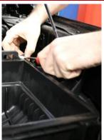
Disconnect wiring harness from lower half of factory air box by using a trim removal tool on the wire clips.
