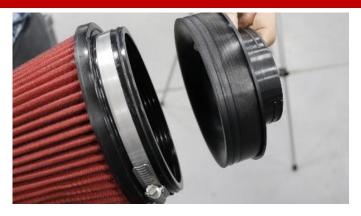
6. Locate filter and filter adapter and insert the filter adapter into filter. Tighten clamp enough that it won't fall off filter but leave loose enough to rotate.
