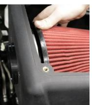
1. Insert the filter into the air box with the adapter side down. Rotate the top of the filter down into the air box and rotate the filter around and push the adapter through air box.
