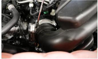
Loosen the clamp securing the factory air duct to the throttle body using a flathead screwdriver or ratchet and 7mm socket.
