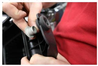
Locate the metal bushing and rubber grommet on side of factory air box and remove both.
