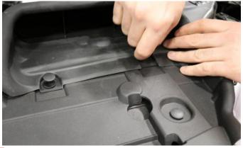
**5.** Locate the air scoop retaining clips from removal step 8 and attach factory scoop.
