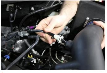
**12.** Connect both vent lines to fittings in air duct.
