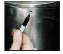
NOTE: IMPORTANT-Make sure that the small drain or weep hole in rear of muffler faces down when muffler is installed.
