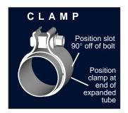
All TORCA clamps should be tightened using a properly calibrated Torque Wrench, Using an air impact gun will damage the clamp and reduce its ability to effectively seal the joint. It may also cause the joint to separate thereby causing damage to your exhaust system and your vehicle.
