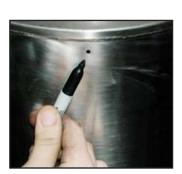
NOTE: IMPORTANT: Make sure that small drain holes in rear of each tunnel muffler face down when installed
