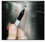
**NOTE: IMPORTANT:** Make sure that small drain holes in rear of each tunnel muffler face down when installed.
