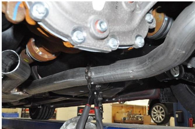
2. Measure 20" away from the flange on the stock resonator, following the outside profile of the exhaust pipe of the passenger side.
