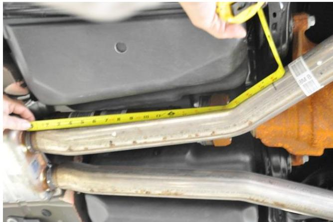
1. Starting on the driver side, measure 19  $\frac{3}{4}$ " away from the flange on the stock resonator, following the outside profile of the exhaust pipe. The tape measure should follow the bend profile of the pipe.
