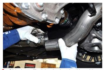
**8.** Slide the muffler inlet pipe into the driver side adapter outlet.
