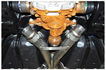
5. Locate the two X-Pipe outlet adapters, and two 3" clamps. Install the clamps on the adapter so that the bolts are vertical with the nuts towards the ground and both bolts are towards the inside of the vehicle when the adapters are installed over the X-Pipe outlets. Tighten the clamps using a ratchet and 15mm deep socket, until the adapters are snug on the pipes.
