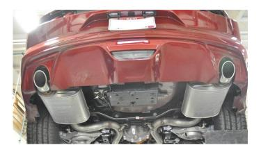
12. Adjust the system accordingly, including the adapter overlap on the stock exhaust, the rear muffler depth and rotation. Verify the exhaust tips are centered in the bumper valence. Check clearances between the system components and chassis. At this time, tighten all clamps to 45ft-lbs using the torque wrench and 15mm socket.
