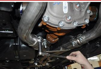
11. Repeat Install Steps 7-9 on the passenger side of the vehicle. Once the exhaust system is secure, it is safe to remove the jack stand from beneath the X-Pipe.
