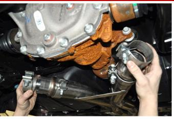
6. Locate two 2½" clamps. Install the clamps on the adapter outlet pipes so that the bolts are vertical with the nuts towards the ground and the bolts towards the outside of the vehicle. WARNING: Do NOT tighten the clamps at this step, as the stock axle pipes will then not be able to fit inside the adapters.
