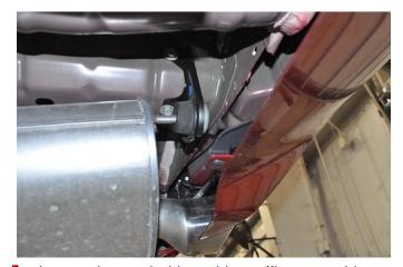
Locate the stock driver side muffler assembly. Slide the rear hanger into the rear hanger grommet located on the vehicle above and just inside of the passenger side tip cut out.
