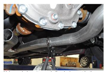
Using a chain cutter or similar device, cut both the driver and passenger side exhaust pipes at the marked locations. Place an adjustable stand or similar device under the stock tunnel section of the exhaust for support. Once the axle pipes are cut, there are no additional stock hangers supporting the tunnel section.
