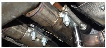
8. Using a 3/8" drive ratchet and 15mm deep socket, loosen the two sleeve clamps at the catback connection point. Both nuts must be loosened in order for the clamp to fully disengage.
