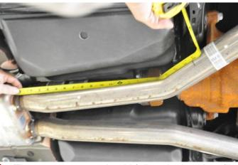
2. The tape measure should follow the bend profile of the pipe.
