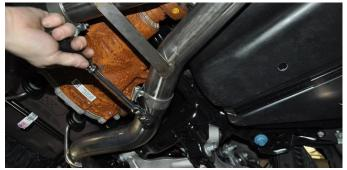
Tighten the clamp connecting the passenger muffler inlet pipe to the passenger side X-Pipe outlet using a ratchet and 15mm deep socket until muffler assembly is snug on the X-Pipe.
