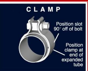
NOTE: Align all clamps so that the center of the clamp bolt is 90 degrees from the notch in the pipe.
