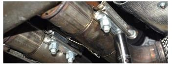
Use a 3/8" drive ratchet and 15mm deep socket, to loosen the two sleeve clamps at the cat-back connection point. Both nuts must be loosened in order for the clamp to fully disengage.
