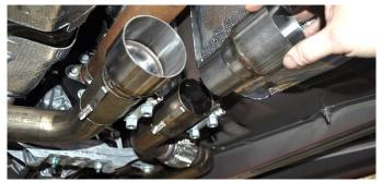
Locate the two X-Pipe inlet adapters. Slide the adapters into the factory sleeve clamps, and tighten using the ratchet and 15mm deep socket, until the adapters are snug in the clamps.
