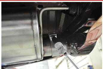
Locate the passenger rear tip assembly and one 3" clamp. Install the clamp on the tip inlet pipe so that the bolt is horizontal with the nut towards the inside of the vehicle and the bolt towards the top. Slide the tip assembly over the muffler outlet pipe and tighten the clamp using the ratchet and 15mm deep socket until the tip assembly is snug on the muffler outlet pipe. Repeat for the driver side tip assembly.
