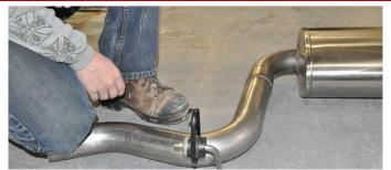
5. Locate the passenger side hanger grommet from Removal Step 5 and the passenger side muffler. Install the hanger grommet onto the front hanger of the muffler in the same position as previously installed on the stock exhaust. NOTE: The use of a soap and water solution may aid in the installation of hanger grommets
