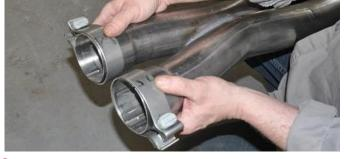
Install two 3" clamps on the driver and passenger inlets of the Double X-Pipe so that the bolts are vertical with the nut towards the ground and the bolts towards the outside of the vehicle.
