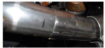
Slide the muffler inlet pipe over the passenger side X-Pipe outlet. NOTE: The use of a soap and water solution may aid in the installation of hanger grommets.
