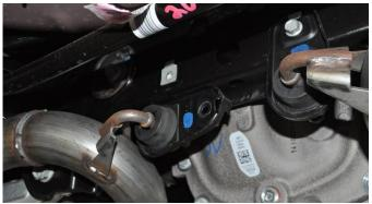
Once the bolt is removed, push up slightly on the exhaust and slide the hanger grommet assembly rearward to free it from the rear suspension subframe. Rotate the hanger grommet assembly a minimum of 90° so that it will not interfere with the rear suspension sub-frame. Save bolt for reinstallation (Install Step 9). Repeat on the passenger side hanger grommet assembly.
