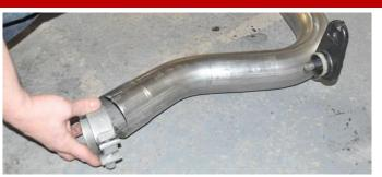
6. Locate one 3" clamp. Install the clamp on the passenger side muffler inlet pipe so that the bolt is vertical with the nut towards the ground and the bolt is towards the inside of the vehicle.
