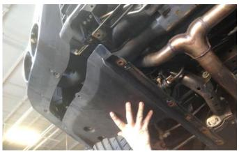
Start on the left side and remove the two larger sized under tray bolts using a 12mm socket and ratchet. Remove the one small bolt with a 10mm socket and ratchet and remove the left side under tray from the vehicle. Set aside in a safe location until reinstalled. Repeat on the right side under tray.
