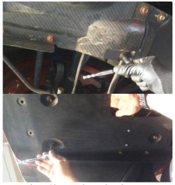
2. Remove the 15 larger sized bolts on the center under tray using a 12mm socket and ratchet.
