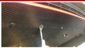
1. Remove the 11 plastic clips on the center and side under paneling with a clip removal tool.
