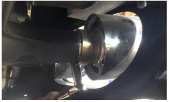
5. Loosen the clamps on the stock tips using a 12mm socket and ratchet. Carefully remove each of the four stock tips from the rear valence.
