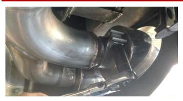
1. Hold the CORSA 5.0" tip with the logo facing up and slide a provided 65mm clamp onto the inlet so the hardware is to the inside of the vehicle, and the nut is downwards.
