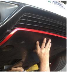
Remove the 8 smaller sized bolts on the center under tray section using a 10mm socket and remove tray from the vehicle. WARNING: Carefully set the center under tray in a safe location until reinstalled.
