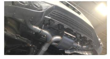
**NOTE:** Immediately following the installation of your exhaust system, you may experience a trace of smoke after initial start-up. DO NOT be alarmed. The smoke is caused by the burning of a small amount of forming oil residue used in the manufacturing process.
