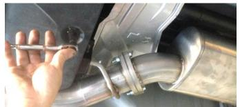
8. Reinstall the bolt from **Removal Step 8** on the center underbody panel closest to the tunnel exhaust hanger using a 12mm socket and ratchet.
