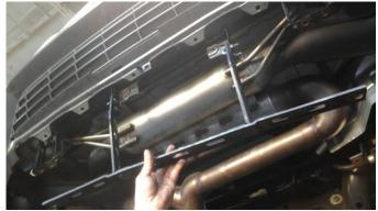
Remove the four nuts securing the rear mounting brace with a 10mm socket and ratchet and remove it from the vehicle.
