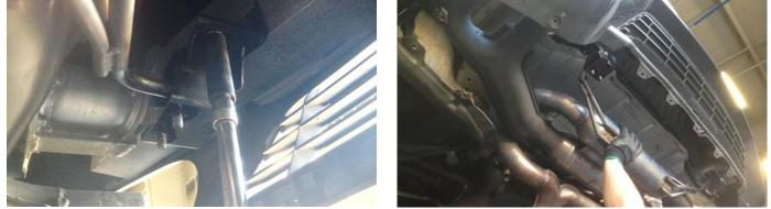
12. The use of a second person is recommended. Remove the two nuts securing each of the exhaust hanger grommets just behind the rear muffler to the chassis using a 12mm socket and ratchet, and a long extension. Carefully remove the rear exhaust section by sliding it rearward off the studs on the front exhaust section. Let the exhaust drop down to free the hanger grommets, then move the entire rear section forward and down to free it from the vehicle. Save Nuts for Install Step 7.
