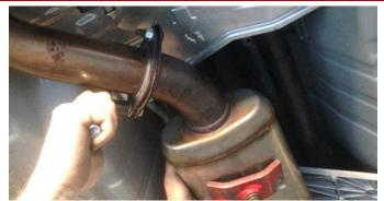
**10.** Remove the two nuts at the center exhaust flange using a 14mm socket and ratchet.
