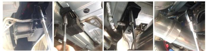
Insert the CORSA rear muffler inlet onto the axle pipe outlet with at least 1.5" of overlap at the slip fit connection. Mount each of the rear hanger grommets to the vehicle's studs in the factory locations using the hardware from **Removal Step 11 & 12**. Tighten the two nuts securing each of the four hanger grommets using a 12mm socket and ratchet, and a long extension. Snug the clamp at the slip fit connection using a 15mm socket and ratchet.
