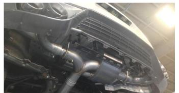
**11.** Visually inspect the exhaust system position, tip alignment, clamp orientation, and exhaust pipe clearance. Make any necessary adjustments at the slip joints and flange connections.
