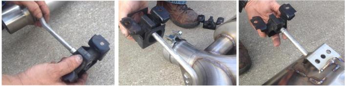
Insert the CORSA rear muffler assembly hangers into the rubber hanger grommets from Removal Step 15 as shown.
