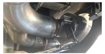
**10.** Hold the CORSA 5.0" tip with the logo facing up and slide a provided 65mm clamp onto the inlet so the hardware is to the inside of the vehicle, and the nut is downwards.
