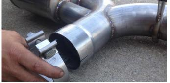
**3.** Pre-assemble the provided 3.5" clamp onto the inlet of the rear muffler assembly with the clamp hardware on the top side of the muffler inlet, and the nut facing towards the muffler case.
