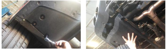
4. Start on the left side and remove the two larger sized under tray bolts using a 12mm socket and ratchet. Remove the one small bolt with a 10mm socket and ratchet and remove the left side under tray from the vehicle. Set aside in a safe location until reinstalled. Repeat on the right side under tray.
