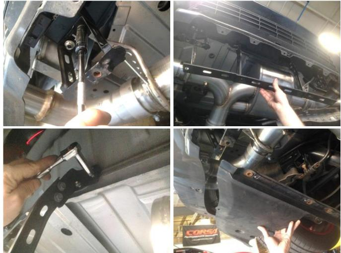
Reinstall all the rear underbody paneling and related bracketry. Refer to Removal Steps 1-6 for more details.
