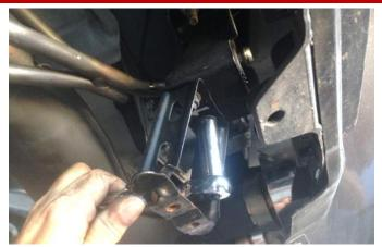
**6.** Remove the 4 nuts securing the left and right mounting braces (2 per side) using a 12mm socket and ratchet, and remove from vehicle.
