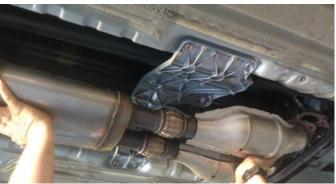
13. Remove the two nuts at each of the front exhaust flanges using a 14mm socket and ratchet, and a long extension. Carefully remove the front exhaust section by sliding it rearward and down off the studs from the stock downpipe to free it from the vehicle.
