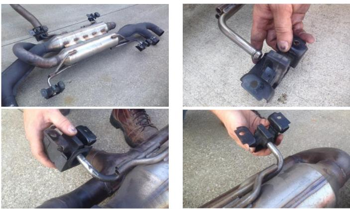
**15.** Now that the cat-back exhaust is on the ground, remove the four rear grommet brackets from the factory hangers using grommet pullers or a similar device. Note the orientation of each hanger grommet before removal, the grommet bracket assemblies are not symmetric and have a front to back offset.
