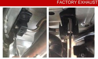
**11.** Remove the two nuts securing each of the exhaust hanger grommets to the chassis just in front of the rear muffler using a 12mm socket and ratchet, and a long extension. **Save Nuts for Install Step 7**.
