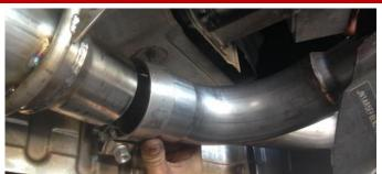
Slide a 3.0" clamp onto each of the CORSA F-Pipe inlets so the clamp hardware sits forward in the vehicle, and the nut is facing downwards.
