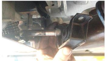
Remove the two nuts securing the tunnel exhaust hanger grommet to the chassis (save for Install Step
