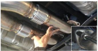
Install the CORSA tunnel muffler assembly onto the downpipe and secure both flanges with the provided M10 flange nuts using a 16mm socket and ratchet. Support the underside of the tunnel muffler with an adjustable support stand.
