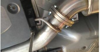
6. Insert the CORSA axle pipe assembly and mount the tunnel hanger grommet to the vehicle's studs using the factory hardware from **Removal Step 9**. Install the supplied 3.5" gasket between the two flanges. Tighten the two sets of provided M10 bolts and nuts at the flange connection using a 15mm socket and 16mm wrench. Tighten the two nuts securing the hanger grommet using a 12mm socket and ratchet, and a long extension.
