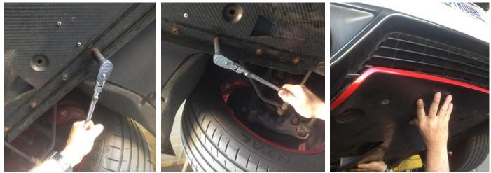
**3.** Remove the 8 smaller sized bolts on the center under tray section using a 10mm socket and remove tray from the vehicle. **WARNING:** Carefully set the center under tray in a safe location until reinstalled.
