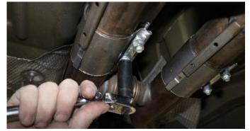
2. Using a 15MM socket or wrench, loosen the factory sleeve clamps (4 Bolts) after the H-Pipe assembly.
