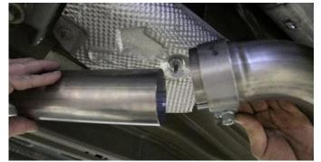
Add a 2.75" clamp to each of the CORSA X-Pipe inlets. Insert the CORSA Inlet Elbow Pipes into the X-Pipe inlets. Snug connection using a 15mm socket or wrench.
