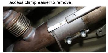
On the driver side, use a flat screwdriver to pry the clamp spring clip from the retainer pin on the H-Pipe repeat on passenger side.
