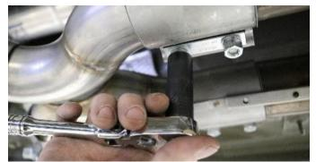
Install the outlet of the CORSA X-Pipe assembly into the factory sleeve clamps at the inlet of the axle pipes. Using a 15MM socket or wrench to snug the 2 bolts on the sleeve clamp. Repeat for opposite side
