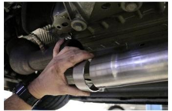
**5.** Adding a 2.75" clamp to the inlet side of each CORSA Inlet Elbow Pipe.
