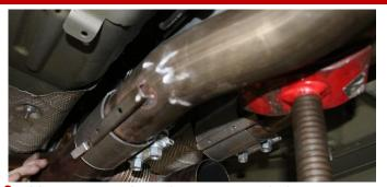
2. You may need another person to help support the X-Pipe and keep it from drooping, so the exhaust does not damage the tip cutouts in the factory rear valance.
