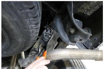
Use grommet pullers to remove the tail pipe hanger near the tip.
