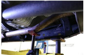
2. Support the front of the system using a jack stand or similar device.
