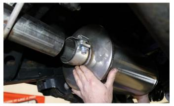
Locate a 3.0" clamp and the CORSA muffler assembly. Install the clamp on the inlet end of the muffler assembly, then slide the expanded inlet end of the muffler assembly over the outlet end of the head pipe. Snugly tighten the clamp using a 15mm socket and 3/8" drive ratchet.
