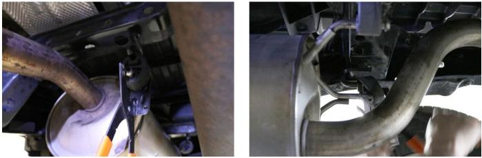
**3.** Using a soap and water solution spray all four factory hanger grommets. (3 near muffler, 1 on tail pipe near exit).
