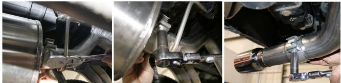
5. Ensure the exhaust system is adjusted properly. Make sure all hangers have clearance, the tailpipe is not contacting the rear axle or chassis, and the tip is adjusted to preference. Begin at the front of the vehicle and fully tighten all bolts and clamps using a torque wrench. Tighten the bolts securing the flange using a 14mm socket to 22 Ft-Lbs, the three 3" clamps to 45 Ft-lbs using the 15mm socket.
