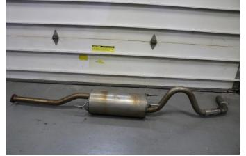
**5.** Carefully remove the factory exhaust system from the vehicle by pulling the exhaust system forward through the chassis, rotating it as needed to clear the suspension, rear axle, and spare tire.
