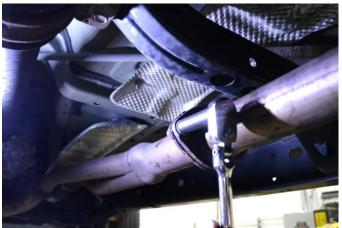
Loosen and remove the two retaining bolts that secure the muffler inlet flange using a 3/8" ratchet and a 14mm socket. The bolts will not be reused.
