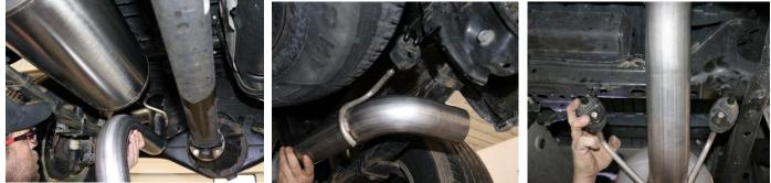
3. Install a 3.0" clamp on the inlet end of the CORSA tail pipe assembly, then feed the tail pipe over the rear axle in the vehicle. Insert the front and rear hangers into their corresponding rubber grommets, slide the expanded inlet end of the tailpipe onto the outlet end of the rear muffler. Adjust the tailpipe so the outlet end is parallel and level with the ground. Snug clamp using 15mm socket and 3/8" drive ratchet.
