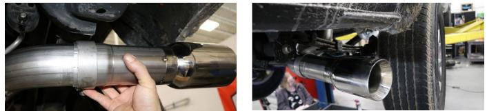
Locate the last 3.0" clamp and the CORSA tip assembly. Slide the clamp over the expansion and then slide the expanded end of the tip assembly onto the tail pipe outlet. Adjust rotation of tip until the CORSA logo is facing upwards. Snugly tighten the clamp using a 15mm socket and 3/8" drive ratchet.
