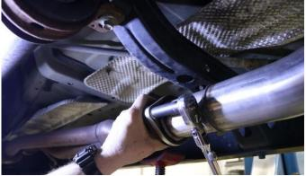
Locate the two supplied M10 bolts and CORSA head pipe assembly. Verify that the factory flange gasket is in place. Insert the head pipe hanger into the factory grommet, then align the head pipe flange with the stock flange, and secure with the supplied bolts. Tighten the bolts with a 14mm socket and 3/8" drive ratchet.
