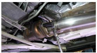
**3.** Use a 15mm socket (or wrench) to snug the Flange Nuts, but do not tighten. Tightening now may hinder proper alignment of the entire system. These will be torqued later.
