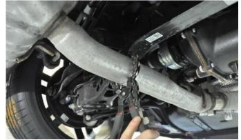
5. Using the Chain Style Pipe Cutter, cut both the Driver and Passenger Factory Exhaust pipes at the marked locations. The Factory Muffler will remain supported by the Muffler Grommets.
