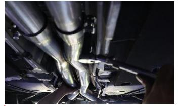
6. Locate the Double X-Pipe and 2 Clamps. Slide a Clamp over each front leg of the X-Pipe so that the nuts on the Clamps will located on the outside of the X-Pipe and face down, as shown in the next step. Slide the X-Pipe flared ends over the Drive and Passenger Head Pipe Adapters. The rear of the X-Pipe will need to be supported by a Jack Stand or similar until the Rear Adapters are installed.
