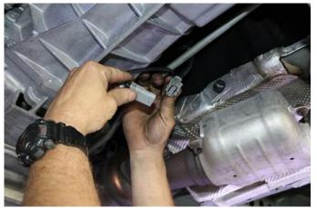
2. Carefully unclip the Passenger-side O2 sensor plug from the wiring harness.
