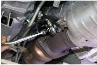
Remove the Passenger-side O2 Sensor from the Stock Head Pipe with a 7/8" O2 Sensor Socket (or 7/8" Open-end Wrench), and store it in a safe location.
