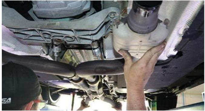
**10.** With assistance, push the Factory Crossover Pipe rearward to remove Driver-side adapter from the Factory Sleeve Clamp. This may require Penetrating Lubricant Spray to release the Adapter from the Clamp. After the Adapter Pipe is released, lower the Factory Crossover Pipe and remove from under the car.
