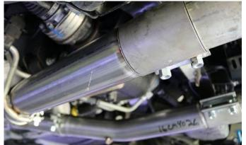
Note: If you are installing a CORSA Axle Back kit, complete its installation before continuing. When the CORSA Axle Back kit is installed, resume this installation. Slide the Sleeve Clamps over the compressed end of the Rear Adapters.
