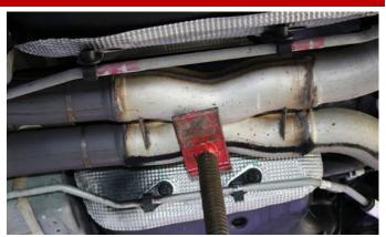
**6.** Support the Factory Crossover Pipe using a jack stand or similar device.
