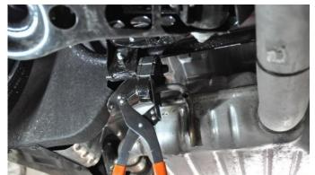
Note: If you are installing a CORSA Axle Back kit, skip this step and refer to Steps 3 and 4 in the Removal section of the CORSA Axle Back instructions. Remove the two Hangers on the rear each side from the Factory Grommets using the Exhaust Hanger Removal Pliers or a similar device. <u>Note:</u> Careful not to damage the Grommets during removal. (Will be reused during installation)
