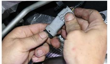
**16.** Reconnect the Passenger-side O2 sensor wiring harness plug.
