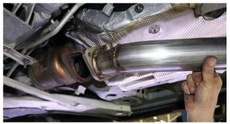
**1.** Locate new Passenger-side Head Pipe Adapter and Gasket. Place the Gasket over the studs, slide the Head Pipe Adapter over the studs.
