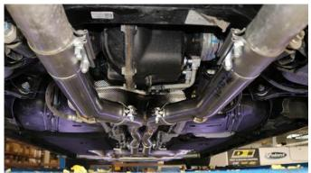
Once the entire exhaust system is properly adjusted, tighten all clamps to 45ft-lbs (61Nm) using the torque wrench and 15mm socket.
