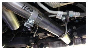
Next, rotate the Rear Adapter Pipe and slide the flared end of the Rear Adapter over the rear leg of the Double X-pipe. Do <u>not</u> slide the Sleeve Clamps on at this time. INSTALLATION INSTRUCTIONS
