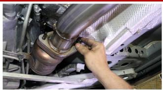
While holding the Head Pipe Adapter (or with assistance), start the Factory Nuts onto the studs
