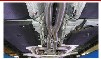
Now adjust the entire exhaust system. Ensure the adapter overlaps, the rear tip depth and rotation so that the tips are centered and aligned. Check the position of all hangers to make sure they are properly seated within their corresponding grommets. Check clearances between the system components and chassis.
