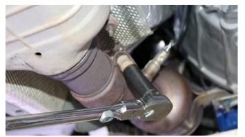
On the Driver side, locate the Factory Slip Clamp at the rear of the Catalytic Converter. Use a 15mm socket (or wrench) to loosen the nut on the Slip Clamp. Do not fully remove the nut!
