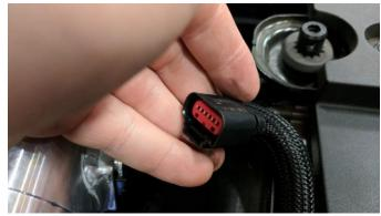
On the driver side, locate the harness connector for the mass air flow sensor. Release the red security clip by pulling the red clip toward the wires and then disconnect the wires from the sensor.
