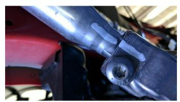
Reinstall the steering shaft from Removal Step 14 to the universal joint using a ratchet and a T40 Torx bit socket.
