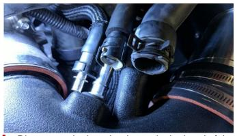
4. Disconnect the breather hoses in the bend of the intake duct using pliers to loosen the hose spring clamps. The third hose has a button-style clamp. Press the release buttons and carefully pull the hose off the barb. Aftermarket intake shown in picture for reference only.
