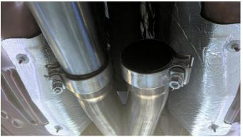
**15.** Install one of the donut gaskets on the passenger side header collector. Insert the outlet elbow into the inlet side of the CORSA X-Pipe.
