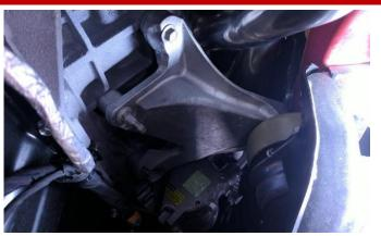
10. Reinstall the factory engine mount brackets using a ratchet and 13mm socket. Passenger Side: Ensure the top bolt in the front has a threaded stud on the hex end. Reinstall the ground strap and secure with the 15mm nut removed during Removal Step 17. Lower the engine back onto the engine mounts.
