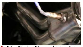
Reinstall the front O2 sensors into the collectors. WARNING: The sensors are fragile and sensitive to contamination, take care when handling. Tighten them using an O2 sensor socket and ratchet or a 22mm wrench. PRO TIP: The best way to secure the passenger side sensor is to route the sensor plug behind the black tape-wrapped transmission sensor wire near the starter.
