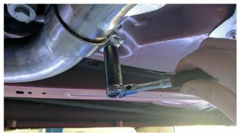
20. Begin the final alignment process by snugging all clamp bolts using a ratchet and 15mm socket. Align the adapter pipes so they are roughly parallel to the ground and running straight toward the rear of the vehicle. The pipe overlap between the elbows and at the inlet side of the X-Pipe should be slightly more than 1.5". With the system snugged, adjust pipe overlaps and check all clearances to heat shields, wiring harnesses, and chassis components.
