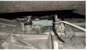
19. Repeat Install Steps 14-17 on the driver side of the vehicle. Driver Side: Remove the harness connector from the transmission and rotate it down so the connector is on the bottom side of the mounting point with the open end facing the rear of the car. Connect the driver side rear O2 sensor.
