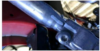
**14. Driver Side:** Remove and **save the two bolts** (save for Install Step 7) securing the steering shaft to the universal joint using a ratchet and a T40 Torx bit socket.
