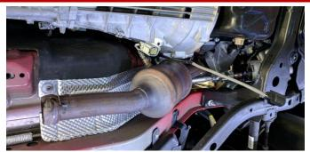
12. On the driver side, loosen the spherical joint clamp near the catalytic converter using a 15mm socket and ratchet.
