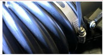
5. Loosen the band clamp around the air inlet tube using a flathead screwdriver or nut driver. Remove the single 10mm bolt securing the box. Save bolt for reinstallation (Install Step 24). Remove the intake box assembly from the vehicle.
