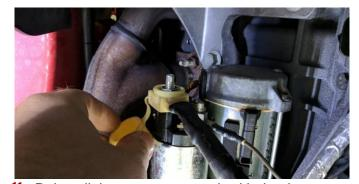
11. Reinstall the starter, secure it with the three 10mm bolts from Removal Step 15 using a 1/4 drive ratchet and 10mm socket with 3" extension. Connect the starter wires using the ratchet with the 10mm and 13mm nuts.
