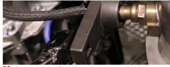
20. Remove the O2 sensors from the factory manifolds and catalytic converters using an O2 sensor socket and ratchet or 22mm wrench. PRO TIP: Label the location of each sensor so they can be installed into the same location within the CORSA Performance headers.
