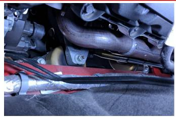
23. Secure the top of the engine mounts with the nuts removed during **Removal Step 6**, using extensions, a ratchet, and a 15mm socket.
