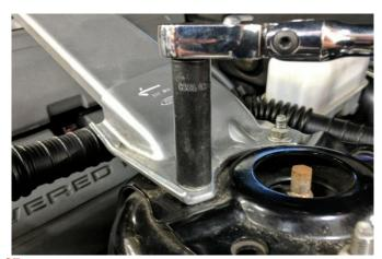
25. Reinstall the engine cover and press into place. Reinstall the strut tower bar, if present, (from Removal Step 2 and secure with the shock mount nuts, 15mm socket and ratchet.
