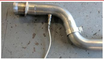
13. Install the rear O2 sensors into the CORSA flanged adapter pipes with O2 bung. The adapter pipes are symmetrical for driver and passenger. Ensure the O2 sensors are installed on the correct side of the vehicle.
