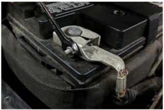
Remove the black negative battery cable using an 8mm wrench.
