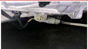
**18.** Connect the passenger side rear O2 sensor to the vehicle harness. (Located on the side of the transmission housing).
