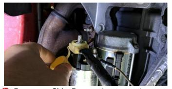
**15. Passenger Side:** Remove the starter wires using a ratchet and a 10mm and 13mm sockets.
