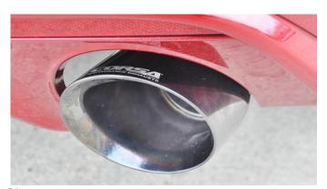
21. The help of a second person is required for this step. Ensure the exhaust tips are properly centered within the rear bumper valence. Tighten all clamps to 45ft-lb. Tighten the spherical flange nuts and bolts to 15ft-lb or 180in-lb using a 1/2" socket, extensions (as necessary), a torque wrench, and 1/2" box wrench.
