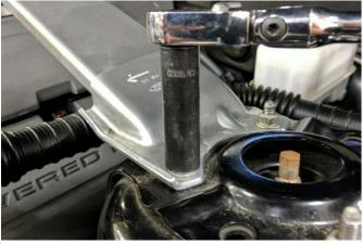
Remove the strut tower bar, if present, using a 15mm socket and 3/8" ratchet. Save for reinstallation (Install Step 25).
