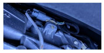
11. Rotate the vehicle harness connector 180 degrees so it points toward the rear before reinserting the "tree" mount into the hole in the transmission housing.
