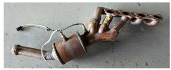
18. Using a 13mm socket and ratchet or ratcheting wrench, remove eight nuts on each side securing the factory manifolds to the heads. (Save nuts to return vehicle to stock). WARNING: Take care when removing the factory manifolds from the vehicle. The O2 sensors are still in place and can be easily damaged.
