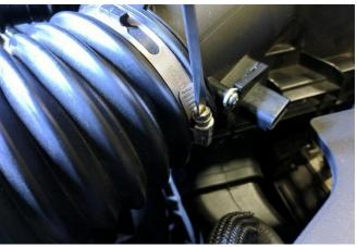
24. In the engine bay, reinstall the air intake box and secure it with the bolt from Removal Step 5.
