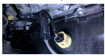
10. Disconnect the driver side front O2 sensor connector located near the oil sensor. Disconnect the rear O2 sensor. PRO TIP: Disconnect the rear sensor connector from its mount in the transmission to remove it.
