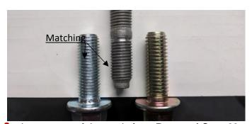
3. Locate one of the studs from Removal Step 23 along with both bags of bolts provided in the hardware kit. Compare the SHORT end threads on the stud to both sets of bolts. Pay close attention to how well they match: One set of bolts is for newer vehicles with coarse threads. The bolts with a fine thread are typically for older vehicles. WARNING: Ensure the threads on the stud match the bolts otherwise serious damage can be done to the engine head.
