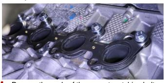
4. Prepare the ends of the correct matching bolts with a small amount of anti-seize lubricant. Locate the multi-layer steel header gaskets in the hardware kit.
