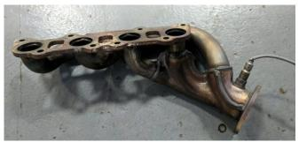
22. Using a 12mm socket and 3/8" ratchet or ratcheting wrench, remove 8 nuts on each side securing the factory manifolds to the heads. (Save nuts to return vehicle to stock). WARNING: Take care when removing the factory manifolds from the vehicle. The O2 sensors are still in place and can be easily damaged. Remove both gaskets from the engine head.
