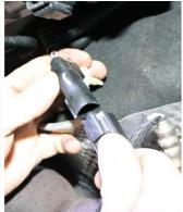
**9.** Disconnect the driver front O2 sensor connector. Disconnect the passenger front O2 sensor connector. (*Automatic Transmission Only*).
