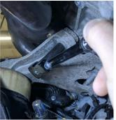
20. Remove the engine mounts from both sides of the engine using a 3/8" drive ratchet (3" extension if needed), 13mm deep and shallow sockets. One bolt on the passenger side is "blind" and has a 15mm nut on it to secure a ground strap to the stud. Save bolt and 15mm nut for reinstallation (Install Step 7).
