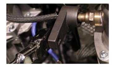
24. Remove the O2 sensors from the factory manifolds and catalytic converters using an O2 sensor socket and ratchet or 22mm wrench. PRO TIP: Label the location of each sensor so they can be installed into the same location within the CORSA Performance headers.
