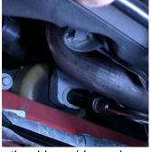
Locate the single nut for the driver side engine mount. Use a 15mm socket, extensions, and 3/8" ratchet to remove the nut. Remove the passenger side nut. Save for reinstallation (Install Step 24).
