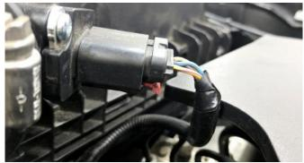
Locate the harness connector for the mass air flow sensor on the driver side and release the red security clip by pulling it toward the wires. Disconnect the wires from the sensor.
