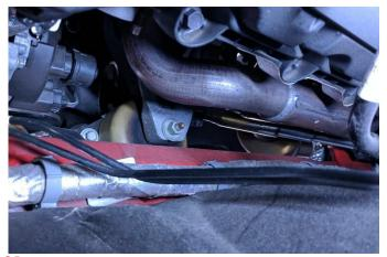
**24.** Secure the top of the engine mounts with the nuts removed during **Removal Step 7**, using extensions, a ratchet, and a 15mm socket.
