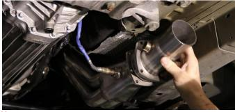
11. Install a CORSA Connection Pipe (Included in Part # 16018) on the passenger side with the O2 bung facing towards inside of the vehicle at a slight upwards angle.
