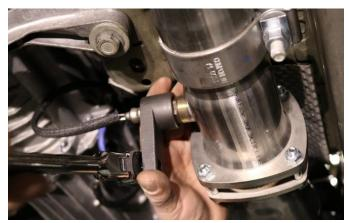
**19.** Tighten O2 sensors using an O2 sensor socket and ratchet or a 22mm wrench.
