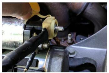
8. Reinstall the starter, secure it with the three 10mm bolts from **Removal Step 18** using a 1/4" drive ratchet and 10mm socket with 3" extension and swivel. Connect the starter wires using the ratchet with the 10mm and 13mm nuts.
