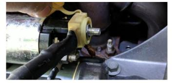
18. Passenger Side: Remove the starter wires using a 1/4" ratchet, a 10mm socket, and a 13mm socket.
