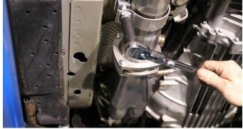
Slide the 2.75" X-Pipe clamp forward and tighten using a 15mm wrench with the nut towards the ground and the bolt toward the outside of the vehicle.
