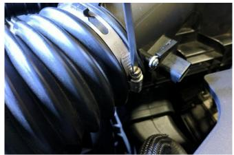
25. In the engine bay, reinstall the air intake box and secure it with the bolt from Removal Step 6. Tighten the hose clamp with a flathead screw driver or nut driver. Connect the airflow sensor cable and lock in place with the red tab. Connect the breather hoses to the intake duct.
