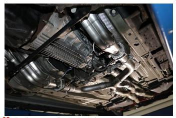
23. Perform one final check for exhaust system clearances to any heat shields or chassis components. Ensure no wires are contacting the headers.
