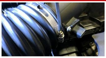
6. Disconnect the breather hoses in the bend of the intake duct by using pliers to loosen the hose spring clamps. Loosen the band clamp around the air inlet tube using a flathead screwdriver or nut driver. Remove the single 10mm bolt securing the box and remove the intake assembly from the vehicle. Save for reinstallation (Install Step 25).
