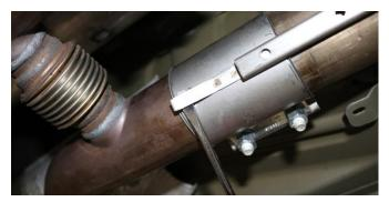
**15.** Use a flathead screwdriver or similar pry device to release the factory sleeve clamp locking clip.
