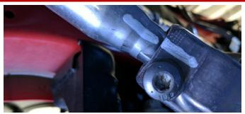
Reinstall the steering shaft from Removal Step
