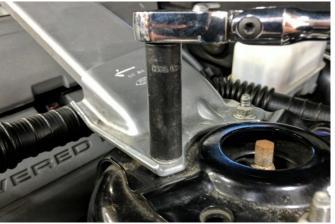
Remove the strut tower bar, if present, using a 15mm socket and 3/8" ratchet. Save for reinstallation (Install Step 26).
