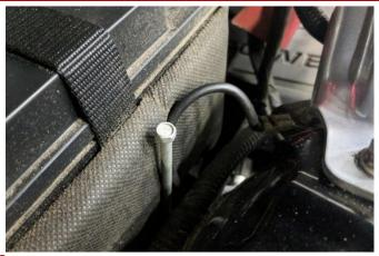
Remove the battery blanket insulation. Loosen and remove the bolt securing the battery to the tray using an 8mm socket and 1/4" ratchet. Save for reinstallation (Install Step 27).
