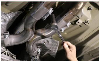
**15.** Tighten the stock sleeve clamp bolts using a 15mm socket and 3/8" ratchet.
