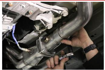
21. Begin the final alignment process by snugging all clamp bolts using a ratchet and 15mm socket. The pipe overlap between all slip fit joints should be slightly more than 1.5". With the system snugged, adjust pipe overlaps and check all clearances to heat shields, wiring harnesses, and chassis components.
