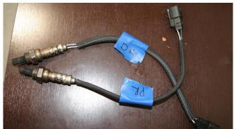
10. Remove the rear O2 sensors and label their positions using a 22mm wrench or O2 sensor socket and 3/8" ratchet. PRO TIP: Label on the connector or the sensor body itself. EXAMPLE: DR for Driver Rear. PF for Passenger Front.
