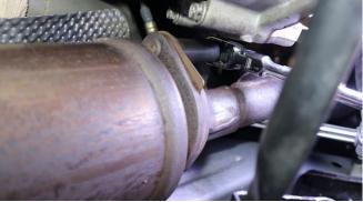
11. Locate the flange connecting the driver catalytic convertor to the manifold. Use a 15mm socket and 3/8" ratchet to remove the last nut. Repeat on passenger side.
