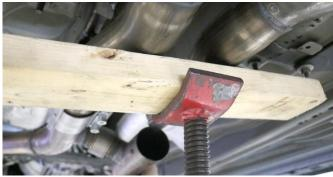
12. Support the factory axle pipes and the driver catalytic converter with a jack stand or similar device. DO NOT let the exhaust droop as it may damage the rear bumper cutouts.
