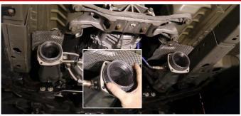
**10.** Install the provided donut gaskets on the collector outlets.
