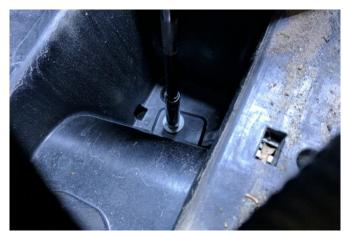
3. Remove battery from the vehicle. Remove the battery tray from the vehicle by removing the three 8mm bolts using a ratchet, long extension, and 8mm socket. Save for reinstallation (Install Step 27).
