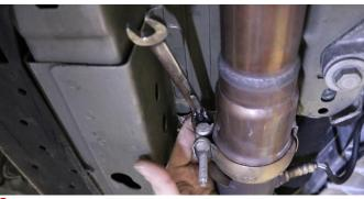
**13.** Loosen the spherical joint clamp on both the catalytic converters using a 13mm wrench.
