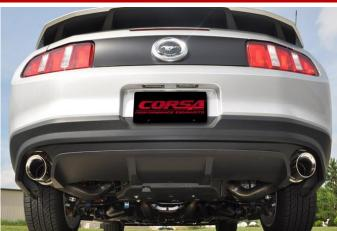
22. The help of a second person is required for this step. Ensure the exhaust tips are properly centered within the rear bumper valence. Tighten all clamps to 45ft-lb. Tighten the spherical flange nuts and bolts to 15ft-lb or 180in-lb using a 1/2" socket, extensions (as necessary), a torque wrench, and 1/2" box wrench.
