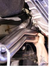
5. Lift one of the headers up and slide the 4 top bolts into the header flange to align to the engine. (This step is much easier with the help of another person). Start the bolt along the bottom of the flange to hold it in place. Start the remaining header bolts by hand to ensure they are not cross-threaded.
