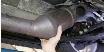
14. Push the entire exhaust system rearward in the vehicle to gain enough space to remove the catalytic converters.
