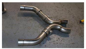
13. Pre assemble the CORSA X-Pipe (Part # 14370 or 14421). Snug two of the 2.75" clamps with the nut towards the ground and the bolt toward the outside of the vehicle. Slide the other two 2.75" clamps onto the inlet pipes before raising the X-Pipe assembly up. NOTE: Install and align clamps according to WARNING box on page 9.
