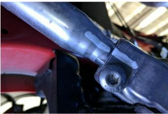
17. Driver Side: Remove and save the two bolts (save for Install Step 9) securing the steering shaft to the universal joint using a ratchet and a T40 Torx bit socket.
