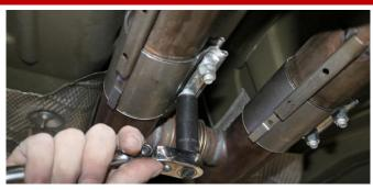
**16.** Loosen the sleeve clamps near the factory intermediate pipe using a 15mm socket and 3/8" ratchet, then remove from the vehicle.
