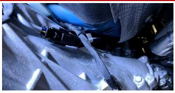
Install the passenger front O2 sensor extension wire. PRO TIP: Route it around the bellhousing at the rear of the engine. This keeps it tucked away from the header once installed.
