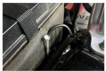
21. Reinstall battery, battery tray, and the battery blanket insulation from Removal Steps 2 & 3.
