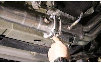
**16.** Tighten the Connection Pipe flange bolts, using a 1/2" wrench and 1/2" socket and ratchet. Torque bolts down evenly and continue sequence until connection is full sealed and no bolts rattle.
