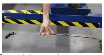
**8.** Locate the flange connecting the passenger catalytic convertor to the manifold. Remove the top nut using three 12" long 3/8" extensions, 3/8" impact swivel, and deep 15mm socket.
