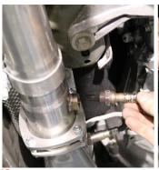
Reinstall the rear driver and passenger O2 sensors, into the CORSA Connection Pipes.
