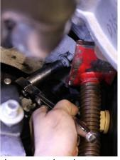
7. Reinstall the factory engine mount brackets using a ratchet and 13mm and 15mm socket. Passenger Side: Ensure the top bolt in the front has a threaded stud on the hex end. Reinstall the ground strap and secure with the 15mm nut removed during Removal Step 20. Lower the engine back onto the engine mounts.
