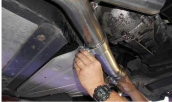
Slide a clamp onto each outlet of the X-Pipe, followed by the appropriate side connection pipe.
