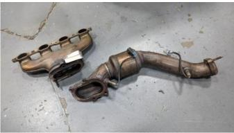
**12.** Remove the six bolts securing the driver side manifold to the head using a 14mm socket and ratchet, or a 14mm wrench. Carefully remove it from the bottom of the vehicle.
