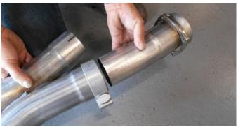
**9.** The CORSA adapter pipes are identical and not side specific. Slide the provided 3.0" clamps onto the inlet side of the CORSA X-Pipe so the clamp bolts face the outside of the vehicle and the nuts are toward the ground. After installing the clamps, slip the adapter pipes into the X-Pipe so the O2 bung faces the outside of the vehicle. [See Double X-Pipe instructions for more specific install details]
