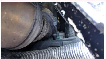
11. Remove the nuts and/or bolts securing the passenger catalytic converter to the exhaust manifold, using a 15mm socket, ratchet, and extensions as necessary. Carefully remove the catalytic converter from the vehicle. NOTE: Take care as the O2 sensors are still in place.
