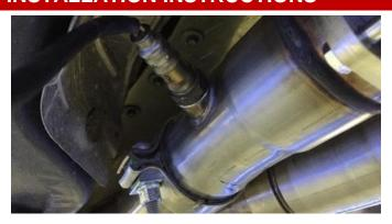
13. Install the rear O2 sensors into the bungs on the X-Pipe adapter elbows. NOTE: The sensors are fragile and sensitive to contamination. Tighten the sensors using an O2 sensor socket and ratchet or 22mm wrench. Plug the sensors in to the appropriate harness extensions.
