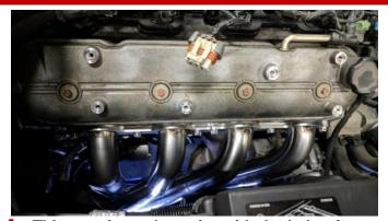
4. This step is made easier with the help of a second person. Lift the header up into the vehicle with the gasket between the header and the engine head. Start the header bolts by hand, ensuring not to cross thread them. Loosely snug the bolts using a 12mm socket and ratchet or 12mm wrench. Repeat Install Steps 3 and 4 on the driver side of the vehicle.
