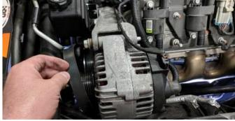
19. Replace the serpentine belt over the alternator. Check that the belt is properly routed through all other pulleys. NOTE: Refer to owner's manual for belt routing. Ensure the grooves and ridges are properly seated in other pulleys and rollers.
