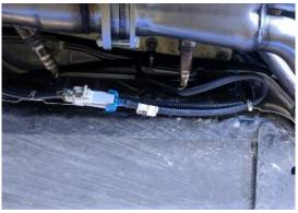
**14.** Use the cushioned "Adel" clamps and metal cable ties included in the hardware kit to secure the loose O2 extension wires up and away from the exhaust. **PRO TIP:** It is easier to remove a bolt or two from the heat shield above the X-Pipe, install the clamp with wire onto the bolt, and then reinstall the bolt.
