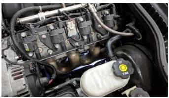
**5.** Carefully remove the passenger and driver spark plug wires. Remove the spark plugs on both sides using a 3/8" ratchet, 3" extension, and spark plug socket. **NOTE:** Be careful not to break the white ceramic spark plug insulators.
