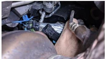
LS7 Z06 Models: O2 sensor wires are most easily accessed from the bottom. Remove the blue locking pin and disconnect the sensor connectors.
