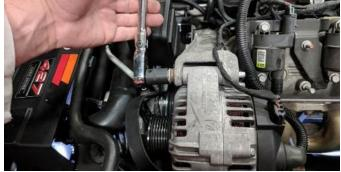
18. Reassembling the components in the engine bay. Begin by replacing the alternator in place and securing with the two bolts from Removal Step 6. Tighten bolts using a ratchet and 15mm socket.
