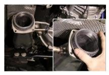
Install the graphite "donut" gaskets onto the header collector outlets with the flat face toward the backing ring on the collector.
