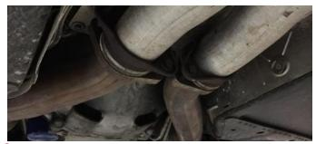
Loosen and remove the nuts securing the X-Pipe to the stock catalytic converter using a 15mm socket and ratchet.
