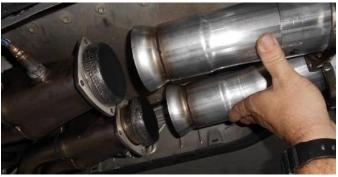
10. This step is easier with the help of a second person. Carefully align the X-Pipe adapters to graphite gaskets. NOTE: The graphite donut gaskets are easily damaged if mating flare pieces are not properly lined up. Lift the X-Pipe into position and adjust the spread/spacing of the slip fit adapters so the flared pipes align with the donut gaskets on the outlet of the header collectors.
