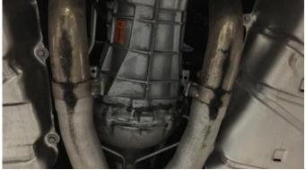
**8.** Loosen the clamps at the rear of the X-Pipe using a 15mm socket and ratchet.
