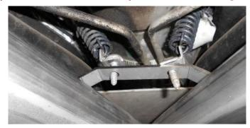
11. Hold the X-Pipe in position on the header collectors and insert the spring hanger studs through the mounting bracket at the rear of the X-Pipe. Thread the nuts from Removal Step 10 onto the studs. Tighten the nuts using a ratchet, appropriate extension, and 13mm deep socket.
