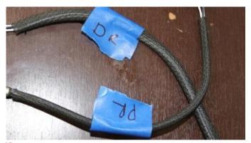
14. Remove the O2 sensors using a 22mm wrench or an O2 sensor socket and ratchet. Label each sensor. Example: "DF" for "driver front" or "PR" for "passenger rear".
