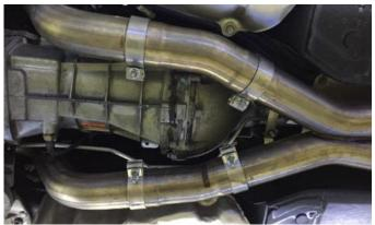
**16.** Insert the muffler axle pipes into the connection pipes. Snug all clamps using a 15mm socket and ratchet, just enough to hold the system in place but still allow them to be adjusted.
