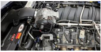
6. Remove the two bolts securing the alternator to the bracket using a 15mm socket and ratchet.
