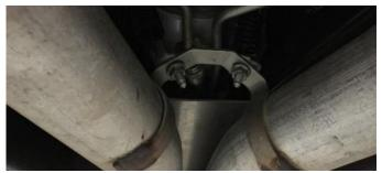
10. Loosen and remove the nuts securing the X-Pipe to the spring hanger near the rear differential using a 13mm socket, extension, and ratchet. Carefully remove the factory X-pipe from the vehicle. NOTE: DO NOT let the exhaust droop as it may damage the rear bumper. Save nuts for Install Step 11.
