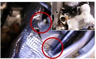
**14.** Remove the remaining 2 bolts on the starter's heat shield using a 13mm socket. Save heat shield and 3 bolts for **Install Step 5**.
