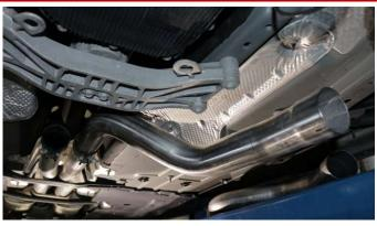
**15.** Slide outlet end of bent connection pipes (18LC4040 and 18LC4041) into the inlets of X-pipe.
