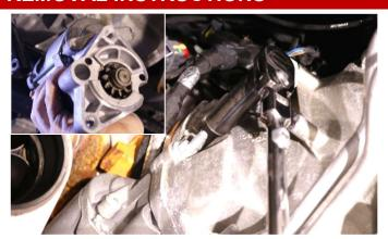
17. Unbolt and remove the starter using a 15mm socket and ratchet. Save bolts for Install Step 5.
