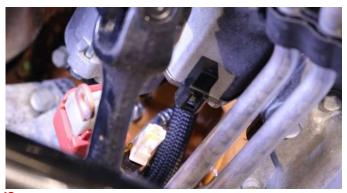
**16.** Unplug the wiring harness from the starter.
