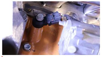
Reinstall the knock sensor to the driver side engine block using a 13mm socket and ratchet. Reinstall the heat shield from Removal Step 18.
