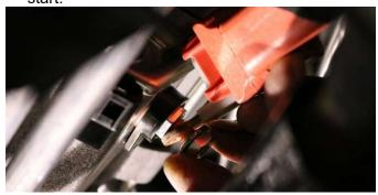
Attach the positive cable to the starter using a 12mm wrench. Plug in the wiring harness to the starter.
