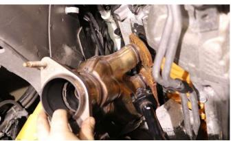
19. Remove the upper and lower driver side factory manifold bolts using a 10mm socket or wrench. Remove driver factory manifold from vehicle. PRO TIP: Remove middle two upper bolts first for easier access. It may be easier to access some of the manifold bolts from engine bay instead of underneath the vehicle.
