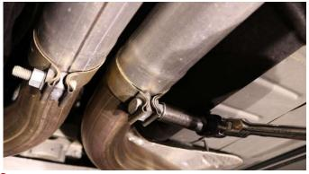
**8.** Using a 15mm socket, loosen the two nuts on the factory X-Pipe inlet.
