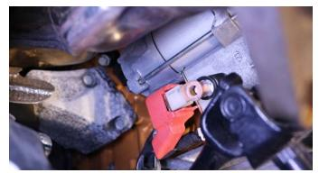
**15.** Unbolt the red (positive) cable on starter using a 12mm wrench.
