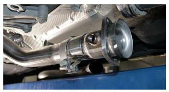
**16.** Add supplied clamp and flange adapter (20MU4171) to inlet of bent connection pipes (18LC4040 and 18LC4041). Rotate upwards until even with donut gasket.
