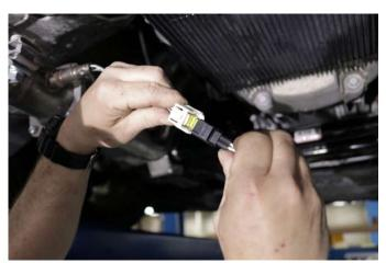
21. Locate the supplied zip ties and supplied driver rear O2 extension cable. Plug the O2 extension into the driver O2 harness and the other end into the O2 sensor. Tuck away any slack from any hot or moving parts.
