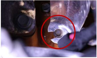
**13.** Remove the 8mm bolt on the starter's heat shield using an 8mm socket and ratchet. Save for **Install Step 5.**
