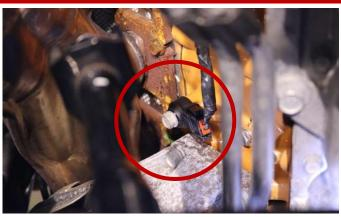
**18.** Remove the knock sensor from the driver side of engine block using a 13mm socket and ratchet.
