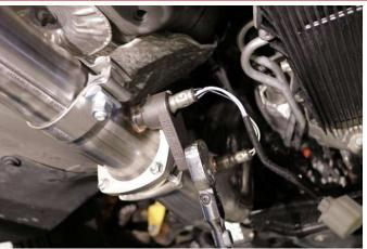
20. Insert and tighten both driver and passenger rear O2 sensor using an O2 sensor socket and ratchet or 22mm wrench. WARNING: Pay attention to your labels.
