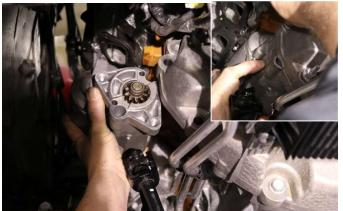
Reinstall the starter using a 15mm socket and the bolts from Removal Step 17. Reinstall the heatshield from Removal Step 14 using the 8mm socket and ratchet.
