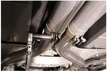
**19.** Tighten the inlet of the X-pipe clamps to factory specifications.
