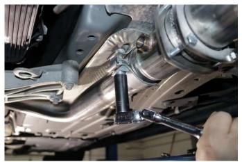
**18.** Tighten supplied clamps to 45 ft-lbs using a 15mm socket and torque wrench.
