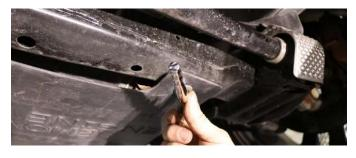
Reinstall plastic bottom engine cover using a 10mm socket and ratchet.
