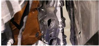
1. Prepare 8 of the supplied header bolts by applying a small amount of anti-seize to each. Insert 4 of the bolts through the lower holes in the provided OEM style stainless steel gasket. WARNING: Hand start each bolt to prevent cross threading. 5.7L Vehicles ONLY NOTE: Driver and passenger gaskets are different. Passenger side has an extra hole for a tube on the front primary. Ensure the gasket is used on the proper engine side!
