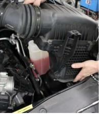
**3.** Disconnect the air intake vacuum tube and remove the factory air intake from the vehicle.
