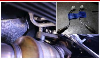
6. Remove the rear O2 sensors and label their positions using a 22mm wrench or O2 sensor socket and 3/8" ratchet. Save them for Install Step 22. PRO TIP: Label on the connector or the sensor body itself. EXAMPLE: DR for Driver Rear or PF for Passenger Front.
