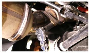
Using a 16mm socket and ratchet or wrench, remove the two nuts on the driver side catalytic converter flange. Repeat on passenger side.
