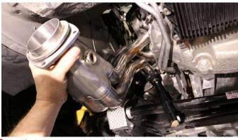
Lift the driver side CORSA header onto the 4 bottom bolts. Start the rest of the header bolts by hand and then torque to approximately 20FT LBS. Note: Gradually tighten all bolts because clearances are tight. Some bolts if left loose and not tightened gradually may contact header primaries if other bolts are fully tightened at the start.
