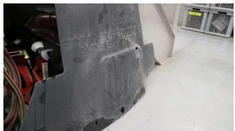
Remove the bottom plastic engine cover using a 10mm socket and ratchet.
