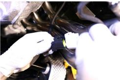
**4.** Insert the passenger front O2 sensor and tighten using an O2 socket or 22mm wrench. Install the supplied O2 extension cable into the front O2 wiring connector and connect the two together.
