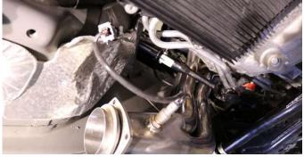
**12.** Tuck away the O2 sensor and extension wires using supplied zip ties and/or vehicle heat shielding. **WARNING:** DO NOT allow wires to contact the headers or other exhaust components.
