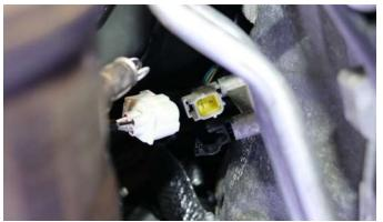
**5.** Unplug the driver and passenger rear O2 sensors from the connectors.
