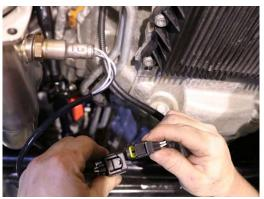
11. Insert the driver side front O2 sensor and tighten using an O2 socket or 22mm wrench. Install the supplied O2 extension cable into the front O2 wiring connector. Connect the O2 wiring harness and O2 extension.
