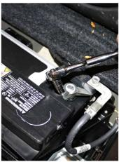
Lift the rear floor mat and the false floor up into the stowed position to allow access to the spare tire and battery compartment. Using a 10mm socket, disconnect the negative battery cable.
