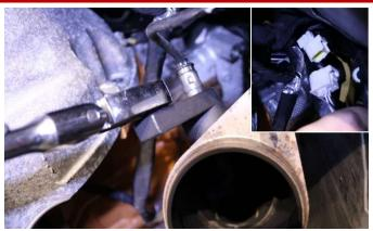
Unplug the front O2 sensor connectors. Remove the O2 sensors from the factory manifolds using a 22mm wrench or O2 sensor socket and 3/8" ratchet. Save for Install Step 4 & 11. PRO TIP: Label each one appropriately for reinstallation.
