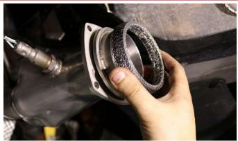
**14.** Install the supplied donut gaskets (99HK7000) to the outlet of the header collector.
