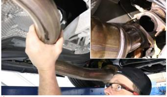
10. Push the entire exhaust rearward in the vehicle to release the catalytic converters from the stock manifolds. Remove catalytic converters from vehicle.
