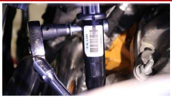
10. Attach the steering shaft using a 10mm socket and bolt from Removal Step 12. WARNING: Pay attention to the marked alignment of the steering shaft.
