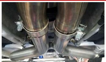
**19.** Slide a clamp onto the front of the crossover pipe with the hardware towards the outside of the car with the nut on the bottom. Slide the non-expanded end into the front of the crossover pipe. Repeat with the other side
