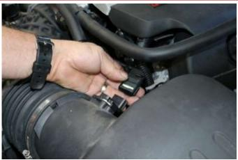
**16.** Plug in the air intake MAF sensor.
