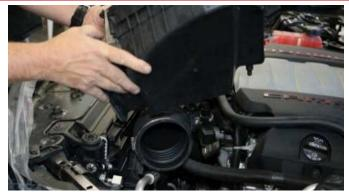
Remove air intake box. Save for re-installation (Install Step # 15)
