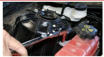
6. To have better access to passenger side of the engine for removal of manifolds, using a 10MM socket or wrench, unbolt and move the coolant reservoir out of the way. It is not necessary to remove the rear hose from it, but you will need to remove the front hose. NOTE: Plug the front hose with a bolt and hose clamp. Put a rubber cap on the nipple of reservoir to prevent coolant loss and leaking during header installation.
