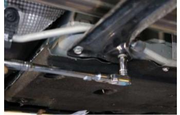
**11.** Using a 13MM socket or wrench remove the center cross brace from vehicle, save for reinstallation (**Install** Step # 11).
