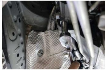
22. Using a 13MM socket or wrench to remove the power wire and two starter bolts. Then remove the starter. Save for re-installation (Install Step # 6).
