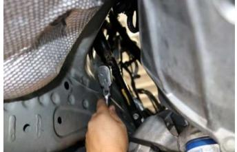
Reconnect the steering shaft with a 11MM socket. NOTE: Make sure to use Loctite or similar on the steering shaft bolt. Tighten the bolts on the driver side header.
