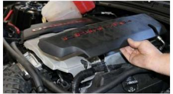
**1.** Remove driver and passenger side engine cover, save for re-installation (Install Step # 13).
