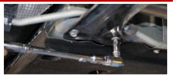
**11.** Using a 13MM socket or wrench reinstall the center cross brace from vehicle **From Removal Step 11**.
