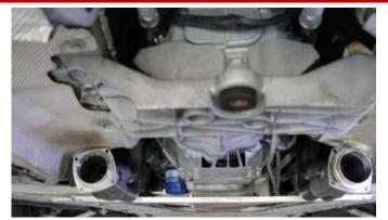
6. Install passenger side header using a 12MM socket or ratchet. PRO TIP: Reinstall starter, starter heat shield, and this side's spark plugs before header is fully tight. From Removal Step 22, 21, & 10.
