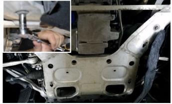
Remove the aluminum K-member brace using a 15MM socket or wrench. Save for re-installation (Install Step # 8).
