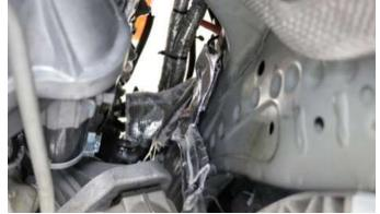
5. On the passenger side of the vehicle, cut and install heat wrap and secure with stainless steel zip ties on the brake line located on the inner frame rail and wiring harness on top of the frame rail.
