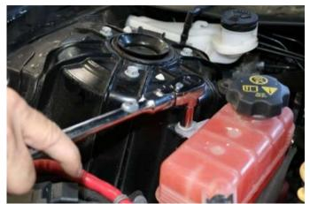
**14.** Using a 10MM socket or wrench, reinstall the coolant reservoir. Make sure to remove your plug and reconnect the front hose. NOTE: Check coolant level and fill as appropriate.
