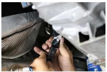
**17.** Reinstall both front o2 sensors on the correct side per your label **From Removal Step 13**. Tighten using a 22mm open end wrench or O2 sensor socket and ratchet. Connect the sensor to the vehicle harness.
