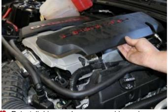
**13.** Reinstall driver and passenger side engine cover **From Removal Step 7**.
