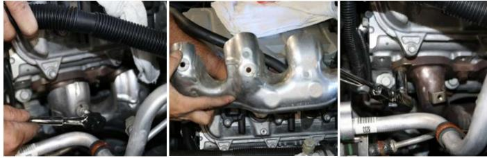
**10.** Use a 5/8 spark plug socket to remove all 8 spark plugs. Save for re-installation (**Install** Step # 4 & 6). **NOTE:** May be easier to loosen and not remove manifold bolts at this time using a 13MM socket or wrench.
