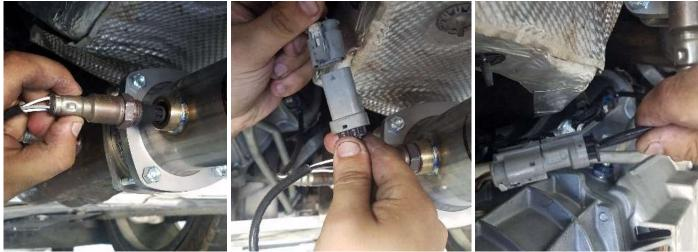
**22.** Re-install the o2 sensors into the bungs. Tighten using a 22mm open end wrench or O2 sensor socket. Make sure that you have the correct sensors in the positions that you labeled them as when you removed them.
