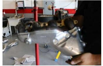
**23.** Using a 13MM socket or wrench, remove factory manifolds.
