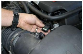
**3.** Unplug the air intake MAF sensor.
