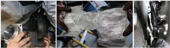
I. On the driver side of the vehicle, install the header and header gasket with just a few bolts using a 12MM socket or wrench. Leave the header loose so the steering shaft can be easily reinstalled and heat wrapped. PRO TIP: Reinstall this side's spark plugs before header is fully tight. From Removal Step 10. Continued on Next Page ...
