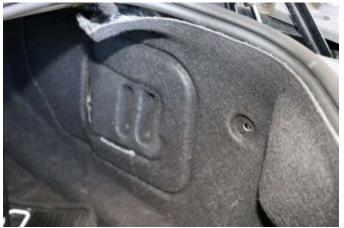
Access the trunk of the vehicle. On the passenger side, locate the battery compartment.
