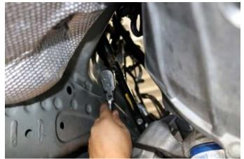
**20.** Using a 11MM socket or wrench unbolt the steering shaft at the top and slide it out of the shaft coming out of the steering column. Move out of the way to make extra room to unbolt the factory manifold. Take care to not turn the shaft as it could cause problems with steering, alignment, and the airbag.
