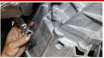
**2.** Install heat wrap around the driver side front and rear O2 sensors wires.
