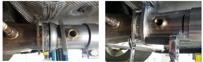
**20.** Make sure that the donut gasket is on the header, then mate the ball flanged end to it. Take care as the donut gaskets can be easily damaged if the flared adapter does not line up properly. Secure them with the bolts and nuts, hand tight. Next, with a ½" socket and wrench, tighten them in a cross pattern so that they clamp down evenly onto the donut gasket. Using a torque wrench, tighten them to 15 ft-lbs.
