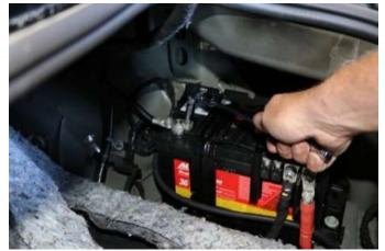
**23.** Using a 10MM socket or wrench, reconnect the negative battery cable from the battery.
