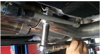
**21.** Snug the clamps at the front and back of the intermediate pipe. Check the alignment and make sure that the pipe is not hanging very low or touching any cross braces or heat shields. Make sure that the crossover pipe is not crooked either, then tighten the clamps from the header back to the crossover pipe.
