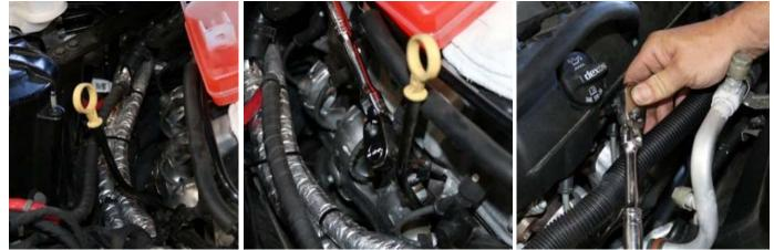
**12.** Reinstall the dip stick mounting bracket, dipstick, and plug wires. Then using a T30 socket, reinstall all coil covers **From Removal Step 8**.
