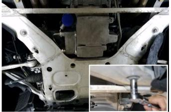
8. Reinstall the aluminum K-member From Removal Step 19.
