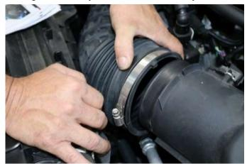
**4.** Using a flat screw driver, un-screw hose clamp from the air duct and remove from intake housing.
