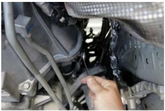
**21.** Use a 10MM socket or wrench to remove heat shield around the starter. Save for re-installation (**Install Step # 6**).
