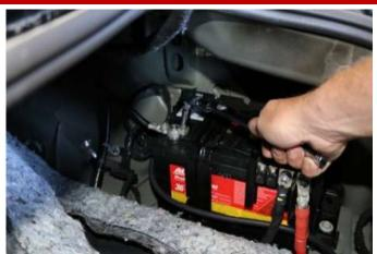
**2.** Using a 10MM socket or wrench, disconnect the negative battery cable from the battery.
