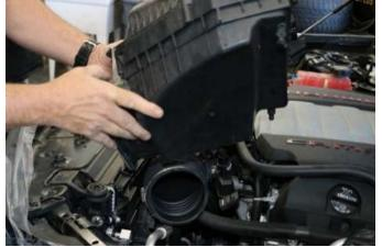
**15.** Reinstall air intake **From Removal Step 5**. Make sure to tighten the clamps on the air ducts.
