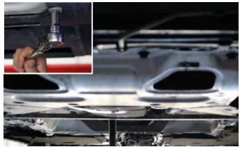
Using 7MM and 10MM sockets or wrenches, remove all plastic covering from underneath the front of the vehicle. Save for re-installation (Install Step # 9).
