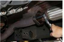
**12.** Remove the two nuts that connect the Y-pipe assembly to the factory exhaust using a 13mm socket or wrench.
