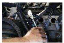
At this point, remove steering column shaft bolt using a 15mm socket or wrench. Replace the steering column shaft bolt and nut with the new nut and bolt supplied with the kit. Replacing the nut and bolt provides an extra margin of clearance between it and the header especially when installing on a 2WD vehicle.
