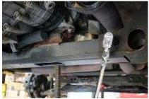
Remove the two-passenger side cross member bolts, one driver's side (the center most) and loosen the other using 21mm socket or wrench. This will allow you to swing down the cross member enough to remove the factorY Y-pipe.
