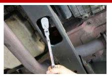
**10.** Remove the two center cross member bolts from the transmission mount using a 15mm socket or wrench.
