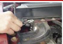
**1.** Remove the negative terminal battery cable using a 10mm socket or wrench.
