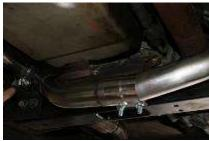
**11.** Install cat delete pipe using (6) 10mm serrated flange nuts. Leave loose do not tighten at this time.
