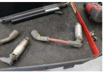
**15.** Re-install spark plugs & wires.
