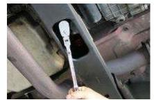
**6.** After headers are in place re-install transmission brace.
