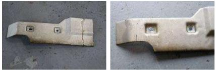
**1**. It may be necessary to trim the shield bolted to the passenger side of the transmission for the y-pipe clearance.
