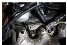
8. The dipstick could be on the driver or passenger side depending on the year. Removal has two possibilities; each requires removing a bolt from the oil dip stick bracket one requires using a 15mm socket or wrench, the other using a T-30 socket. After removing the bolt pull upward gently to remove oil dip stick tube. Temporarily cover dip stick tube hole.
