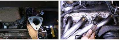
5. Install new header from the bottom of vehicle using care to keep gasket in place. Use a small amount of anti-seize on each bolt making sure to start them by hand to prevent cross-threading. When installing header on the driver's side, the header bolt closest to the firewall may have to be installed from the underside of the vehicle, then install the remainder of the header bolts through wheel well and tighten approximately 20-foot pounds using a 12mm socket or wrench.
