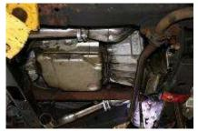
**10.** Slip round spacer on header collector bolts before installing Y-pipes.
