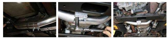
**12.** Install Y-pipe using 2 ½ clamp and 2 ½ band clamp snug clamp do not tighten yet to allow adjustments.
