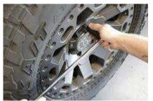
**18.** Re-install front wheels and torque to factory recommendations
