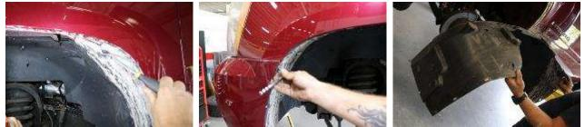
6. Remove wheel inner fender panels from both sides by removing quick release plastic retainers and hex head sheet metal screws using a 7mm socket or wrench. Mark them, if necessary, so that they are replaced in the same position during (re-assembly).
