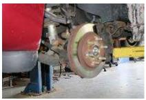
**5.** Remove both front wheels after the vehicle is raised and secure.
