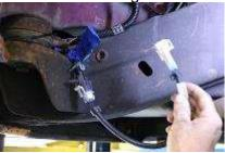
Install the supplied O2 sensor extension for the right (passenger side) front and rear O2 sensor wiring. Slip the connectors together and route the extension cable up and over the right frame rail. Tie this cable up out of the way with the tie wraps.
