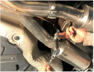
**12.** Make sure to have at least 1.625" of overlap at both slip fit connections. Snug both clamps using a 15mm socket and ratchet, leaving them loose enough for later adjustment.
