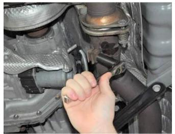
**1.** Using the ratchet and 15mm socket, loosen the clamp in front of the passenger side flange connection.
