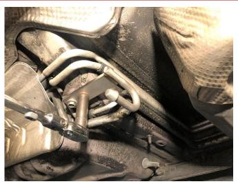
2. Using a ratchet and 13mm socket, install the passenger side hanger assembly with two of the retained bolts at the tunnel muffler location.
