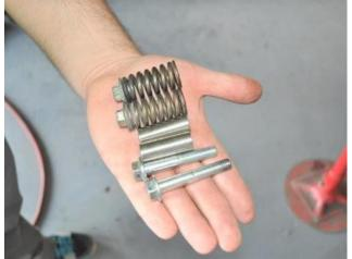
Locate the CORSA driver side tunnel muffler assembly or CORSA tunnel head pipe assembly, the two M10-1.5X60mm bolts and two spacers from the hardware kit, and the two factory springs nut assemblies retained in REMOVAL STEP 2.
