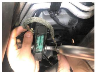
Reinstall the ground clip onto the passenger front hanger of the rear muffler.
