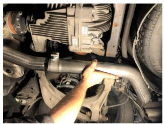
**13.** Locate the CORSA passenger axle pipe assembly and a 2.75" clamp. Position the 2.75" clamp onto the axle pipe inlet, and then install the passenger axle pipe inlet onto the passenger side outlet of the crossover assembly.
