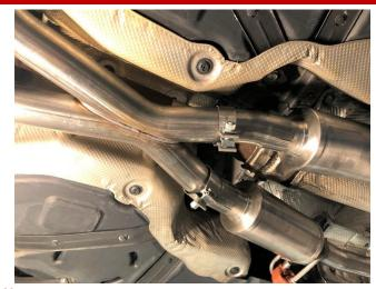
Locate the CORSA crossover pipe assembly and two 2.75" clamps. The crossover pipe is installed with the reinforcement brace towards the ground and towards the rear of the vehicle. Position the 2.75" clamps onto the inlet of the crossover pipe with the clamp hardware facing to the inside and the clamp nuts facing down. Install the crossover pipe inlets onto both tunnel muffler/head pipe assembly outlet pipes.
