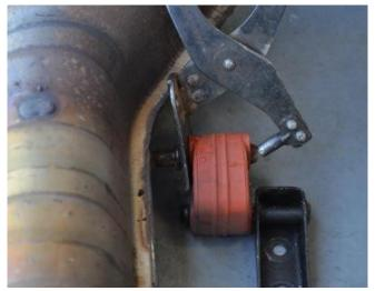
**10.** Using grommet pullers or a similar device, remove both rubber grommets and hanger brackets from the factory tunnel muffler.
