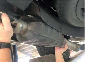
Remove the driver side rear muffler inlet from the axle pipe connection.
