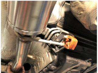
**9.** Locate the CORSA passenger side tunnel muffler assembly or CORSA tunnel head pipe assembly and one of the 2.75" clamps. Position the 2.75" clamp onto the pipe inlet and then insert the passenger side tunnel muffler/head pipe hanger into the rubber grommet.
