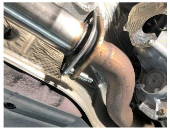
Insert the two supplied M10 bolts (facing forward) through the CORSA driver side tunnel muffler/head pipe flange first, then the stock flange. Next, slide the spacers onto the bolts from the front side, making sure they pass through both flanges as shown.
