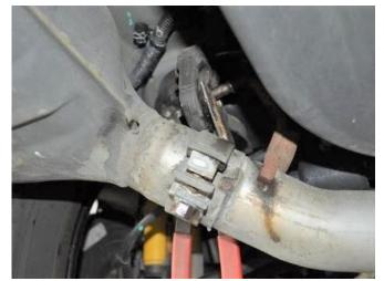
4. Using grommet pullers or similar device, remove the front hanger grommets from both rear mufflers. NOTE: The use of soapy water solution will aid in the removal and later installation of the hangers in the factory grommets.
