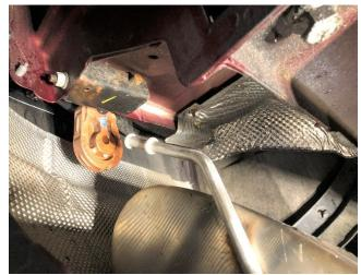
**19.** Repeat **INSTALL STEPS 16-18** to install the CORSA driver side rear muffler assembly onto the outlet of the driver side axle pipe.
