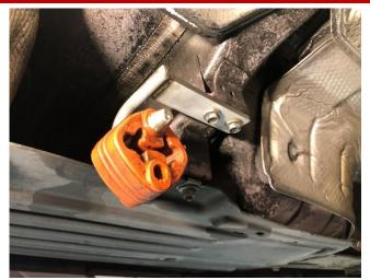
**4.** Repeat **INSTALL STEPS 2-4** to install the hanger assembly on the driver side of the vehicle.
