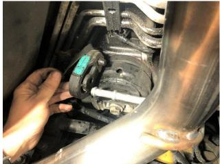
**17.** Insert the forward hanger on the passenger side rear muffler into the rubber grommet.
