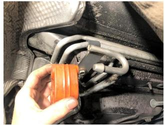
Locate the two factory rubber grommets set aside during REMOVAL STEP 12. Slide one of the rubber grommets onto the hanger.
