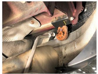
**16.** Locate the CORSA passenger side rear muffler assembly and one of the 2.75" clamps. Insert the rearward hanger on the passenger side rear muffler into the rubber grommet.
