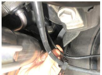
22. Confirm at least a fingertip clearance between the exhaust piping (in front of the rear mufflers) and the wheel sensor wiring for both rear muffler locations. The Sensor wiring can be repositioned and adjusted (if necessary) to create the clearance.
