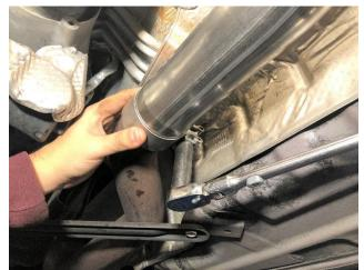
Position the CORSA passenger tunnel muffler/head pipe inlet onto the factory cat outlet, making sure to have at least 1.625" of overlap at the slip fit connection. Snug the clamp using a 15mm socket and ratchet, leaving it loose enough for later adjustment. NOTE: Ensure the CORSA tunnel muffler/head pipe hanger is horizontal while tightening the clamp.
