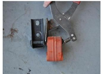
**11.** Using grommet pullers or a similar device, remove both rubber grommets from the hanger brackets.
