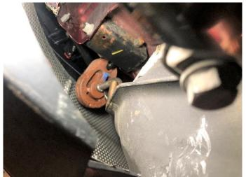
Carefully remove the factory driver side muffler by pulling the rear hanger out of the rubber grommet, then moving the muffler downward to free it from the vehicle.
