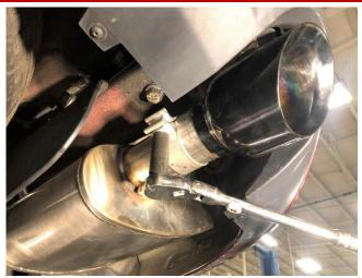
**20.** Locate both CORSA tip assemblies, and two 2.75" clamps. Position a 2,75" clamp onto one of the tip assemblies, and install the exhaust tip onto the passenger side muffler outlet. Adjust the position and rotation of the tip assembly until the tip is centered in the cutout in the rear valence and the CORSA logo is positioned on top of the tip. Repeat this step for the driver side of the vehicle.
