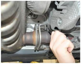
Using the 13mm wrench, loosen the two nuts at the driver side flange location. Set aside the spring nut assemblies to be reused during INSTALL STEP 5.
