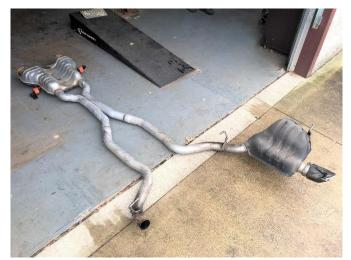
8. The rest of the factory exhaust system will come out in one piece. Pull the rear hanger on the passenger side rear muffler out of the rubber grommet and then slide the entire exhaust system down and rearwards to remove it from the vehicle.
