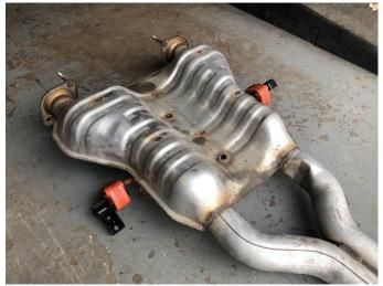
**9.** Locate the factory tunnel muffler, with the factory hanger grommets and brackets still attached.
