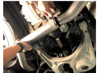
**15.** Repeat **INSTALL STEPS 13-14** to install the CORSA driver side axle pipe onto the outlet of the driver side crossover assembly.
