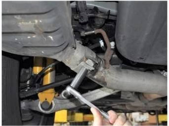
**5.** Using the ratchet and 15mm socket, loosen the clamp on the inlet pipe to the driver side rear muffler.
