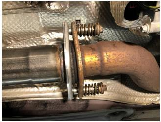
Thread both spring nut assemblies onto the bolts by hand. Using a ratchet with a 15mm socket and 13mm wrench, tighten the flange hardware.
