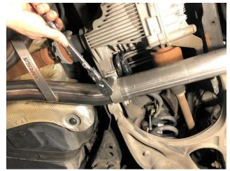
**14.** Make sure to have at least 1.625" of overlap at the slip fit connection. Snug the clamp using a 15mm socket and ratchet, leaving it loose enough for later adjustment.
