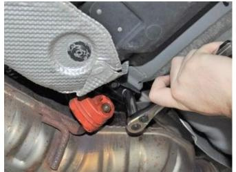
**3.** Using a ratchet and a 13mm socket, remove the two bolts from each hanger bracket at the tunnel muffler location. Set aside the four bolts to be reused during **INSTALL STEP 1.** Remove the ground clip from the passenger side front hanger of the rear muffler
