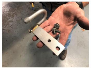
1. Locate the two hanger assemblies provided in the hardware kit, along with the four bolts set aside in **REMOVAL STEP 3**.
