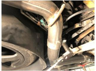
**18.** Position the 2.75" clamp onto the inlet of the passenger muffler assembly, with the clamp hardware facing to the outside and the clamp nut facing down. Install the muffler inlet onto the passenger side axle pipe outlet. Make sure to have at least 1.625" of overlap at the slip fit connection. Snug the clamp using a 15mm socket and ratchet, leaving it loose enough for later adjustment.
