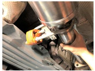
**6.** Insert the driver side tunnel muffler/head pipe hanger into the rubber grommet.
