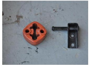
**12.** Set aside the factory rubber grommets to be reused during **INSTALL STEP 3**.
