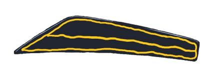
Apply a thin bead of silicone around the perimeter of the insert and a thin bead across the middle as shown above.
