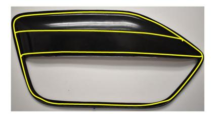
Apply a thin bead of silicone around the perimeter of the insert and a thin bead across the middle as shown above.
