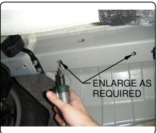
6. Fishwire 1/2-13 x 1 1/4" carriage bolts and SP6 spacers through the enlarged access hole and out the rear-most hole.
