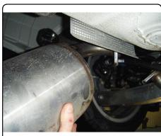
4. Remove heat shields from driver and passenger side. Return heat shields and fasteners to owner.
