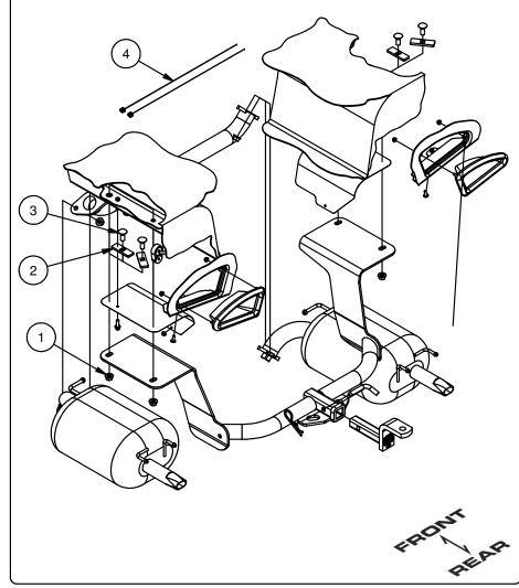
1. Remove exhaust tips from driver and passenger side.
