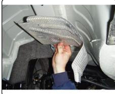
5. Use die grinder to increase the size of the access hole to allow 1/2-13 x 1 1/4" carriage bolts and SP6 spacers to pass through. Use die grinder to increase the rear most hole to allow 1/2-13 carriage bolt to be fishwired through.
