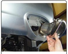
2. Remove rubber isolators from mufflers.
