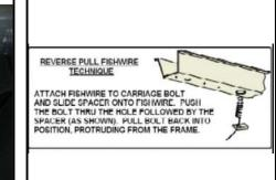
6. Raise hitch over the exhaust and slide it past the exhaust hanger. Secure hitch using 7/16-14 flange nuts. Note: When raising hitch into position you may have to push bolts part way back into the frame to get the plates into position. You may use fishwires to guide hitch during mounting to prevent the loss of bolts and spacers inside the frame rails.
