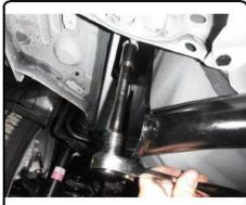
Reinstall rubber isolator (if it was removed in step 1).Installation is complete.
