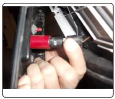
7. Remove the (2) 10mm bolts from under the rear hatch securing the bumper fascia.
