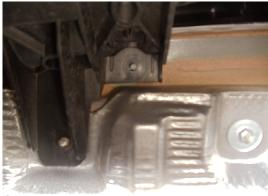
8. To remove bumper cover, gently pull each side of the bumper fascia rearward of the vehicle and set bumper cover aside. (Models with reverse sensors will need to disconnect (4) connectors)
