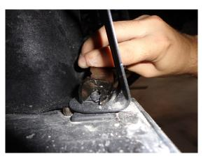
3. Remove (2) 7mm bolts from each side of the wheel well that secure the bumper fascia.
