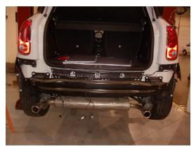
9. Remove the (6) 15mm flange nuts attaching the bumper to the vehicle, remove bumper and set aside.
