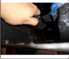
3. Remove (1) plastic rivet each side of the underside of the bumper cover by using a pair of side cutters and cutting off the top of the rivet. Discard removed rivets.
