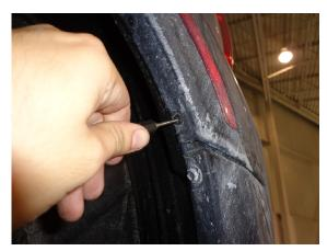
5. Lightly pull the plastic fender flare back on each side exposing an 8mm bolt and the reflector light wiring. Unbolt the 8mm bolt with a wrench and disconnect the reflector light and let hang.
