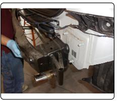
11. Attach hitch to vehicle so that the hitch will be sandwiched between the frame and the bumper. Reuse the 15mm flange nuts on the (6) frame studs to secure the hitch and the bumper. Torque 15mm hardware to 35 lb-ft.
